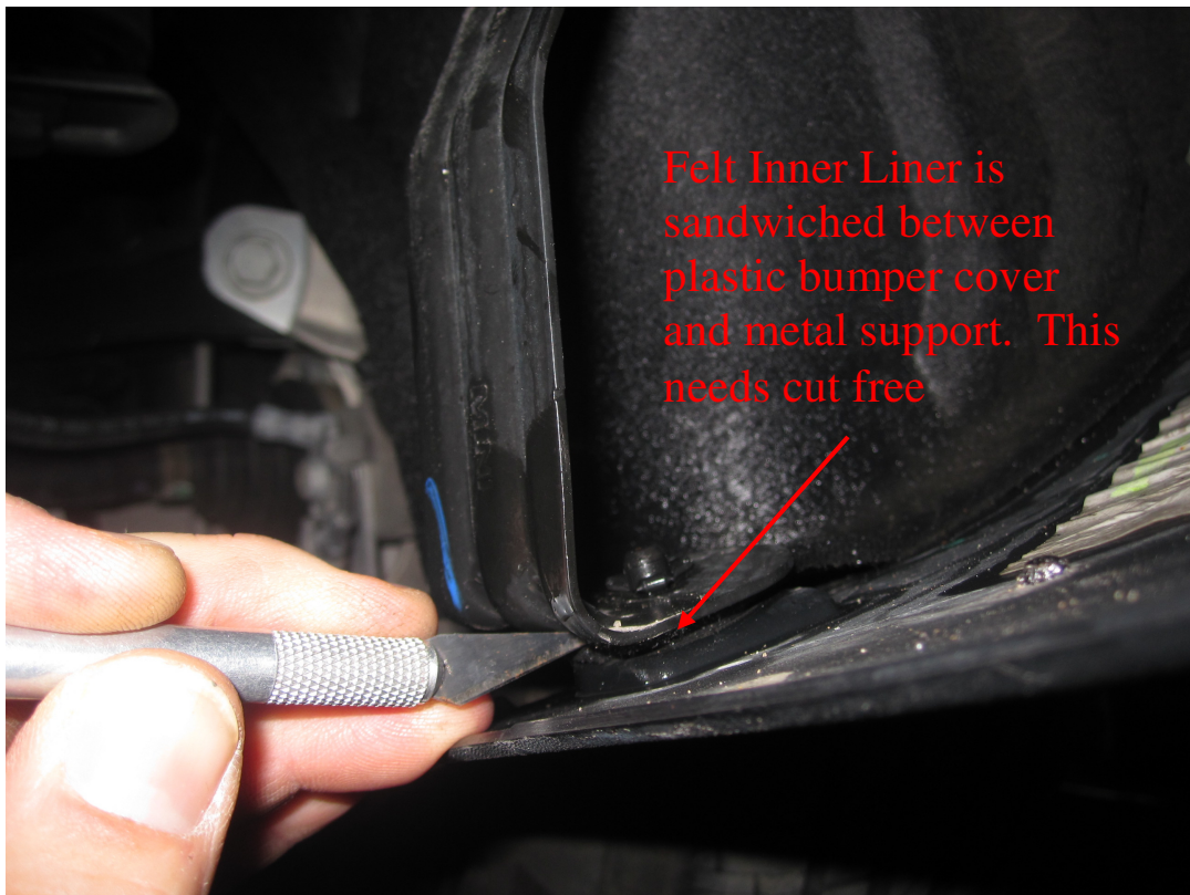
Picture 4 – Trimming the inner liner from the sandwich of the bumper, inner liner, and metal bumper support.
