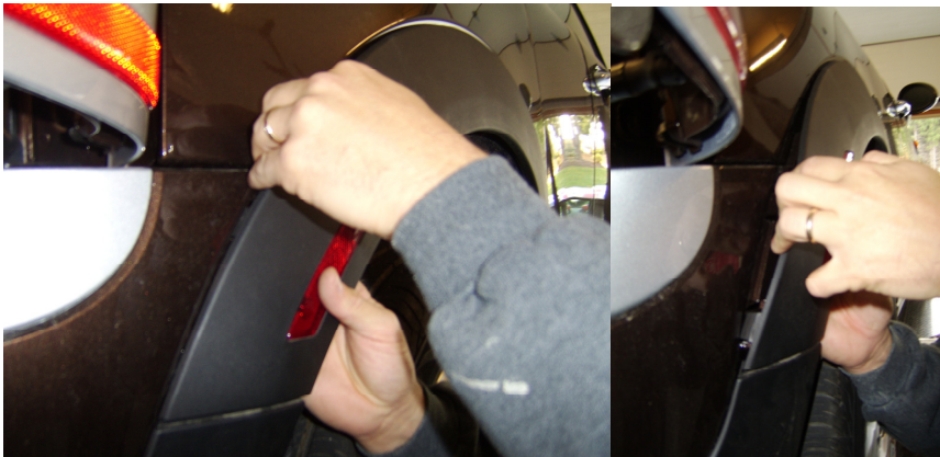
Picture 8 – Accessing hidden fasteners – This photo is of a Clubman, but the process is the same
