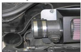
15. Install the provided silicone hose (08756) onto the mass air sensor and secure with the provided hose clamp.
