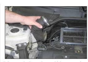
7. Loosen the hose clamp which secures the stock intake hose and then remove the stock intake hose from the vehicle.
