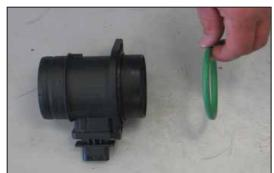
9. Remove the "O" ring from the mass air sensor as shown.
