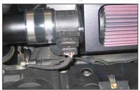
17. Reconnect the mass air sensor electrical connection.
