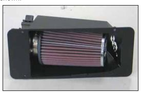
12. Install the K&N® air filter onto the mass air sensor and secure with the provided hose clamp.
