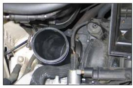
13. Secure the provided silicone hose (08489) onto the throttle body and secure with the provided hose clamp.
