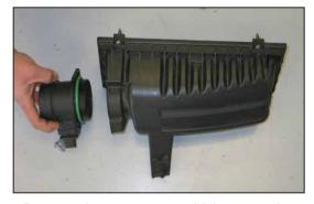
8. Remove the two screws which secure the mass air sensor to the upper air box and then remove the mass air sensor.
