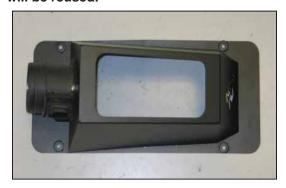
11. Using the provided hardware, secure the factory mass air sensor to the K&N® heat shield as shown.
