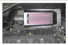
14. Install the heat shield/filter assembly onto the lower air box and secure with the four factory upper air box retaining screws.
