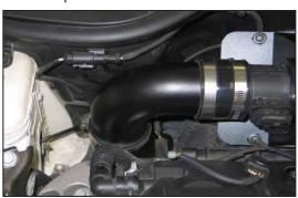
16. Install the K&N<sup>®</sup> intake tube into the silicone hoses and secure with the provided hose clamps.
