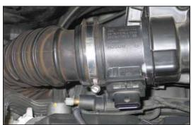
3. Loosen the hose clamp which secures the intake tube to the mass air sensor.
