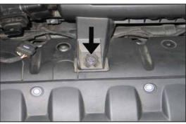
5. Loosen the bolt which secures the upper air box to the valve cover.
