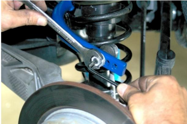
17. Attach end links to NM anti-roll bar using original nuts. Torque to 30 Nm (22 ft-lbs). See adjustment chart for hole mounting information.
