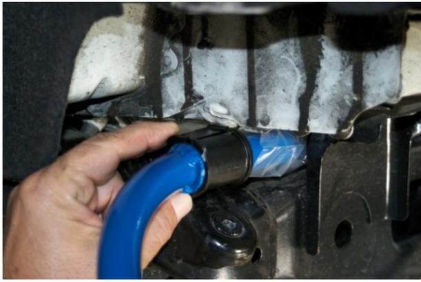
13. Apply supplied grease to inside of supplied bushings and install on the inside of stop washer on NM anti-roll bar.
