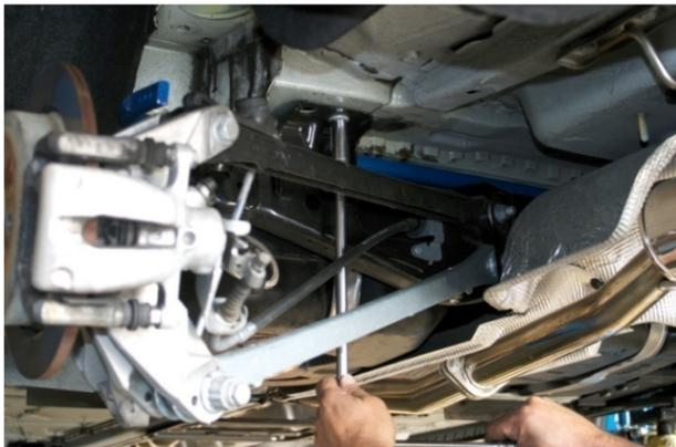
15. Reinstall sub-frame mounting bolts on right-side and torque all [4] bolts to 100 Nm (74 ft-lbs).
