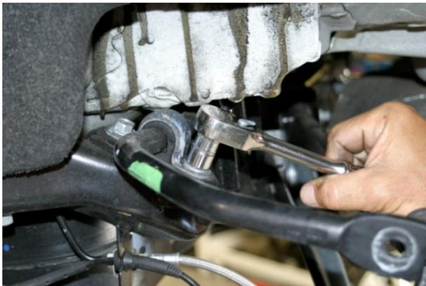
8. Remove the bushing clamp mounting bolts [2] using a 13mm socket. Remove clamp and bushing. Repeat for other side.
