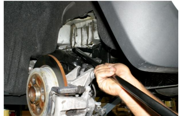
11. Now from left-side of vehicle completely remove original bar.
