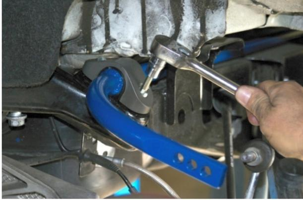
14. Install billet aluminum clamps over bushings and bolt to sub-frame using supplied M8 x 25mm bolts. Torque to 33 Nm (25 ft-lbs).
