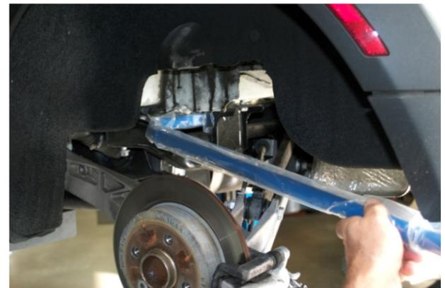
12. Install NM anti-roll bar in reverse of removal of original bar. **HINT:** Leave plastic wrap on bar to protect finish of bar during installation thru sub-frame then remove.
