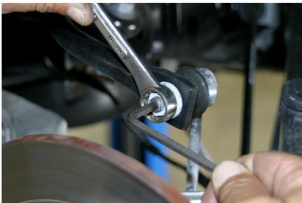
7. Disconnect end-link from original anti-roll bar by securing stud with 6mm hex key wrench and loosening nut with 16mm wrench. Repeat for other side.
