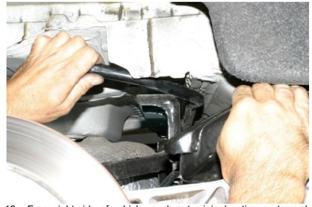
10. From right-side of vehicle, push out original anti-sway toward left-side of vehicle between uni-body and sub-frame.
