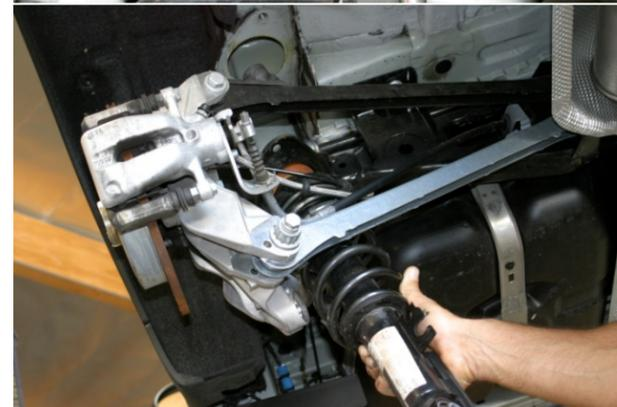
6. Unbolt and remove [2] upper shock mount bolts using 13mm socket and 18" extension. Remove shock and repeat for other side.
