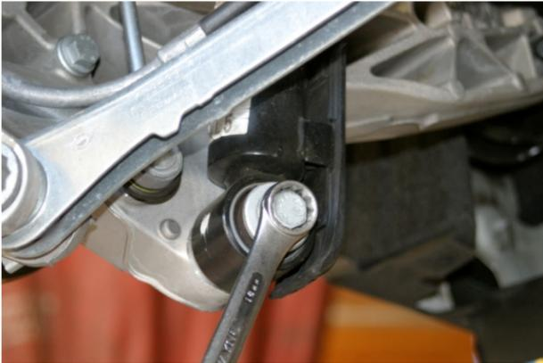
5. Unbolt and remove lower shock absorber bolt using 18mm wrench.
