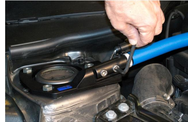
5. Install and tighten all [4] M8 x 20mm hex socket bolts using a 6mm hex key wrench.
