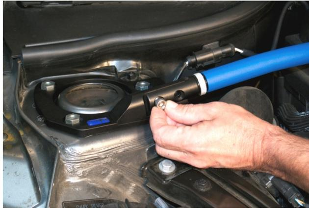
3. Attach NM aluminum tie-bar to base plate on one side at this time with [1] M8 x 20mm hex socket bolts supplied. Do NOT tighten at this time.
