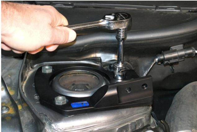
2. Mount and evenly tighten the NM base plate to strut towers using special long-reach nuts – torque to 34 Nm (25 ft-lbs.). **NOTE:** Hand thread all nuts to be certain that shoulder of nut centers into NM base plate holes before torquing.
