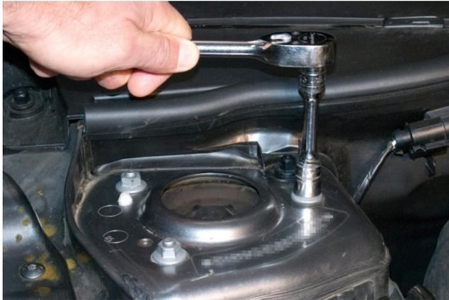
1. Park MINI on a level surface and remove the [6] 13mm hex nuts (3 on each side) on top of the front strut towers
