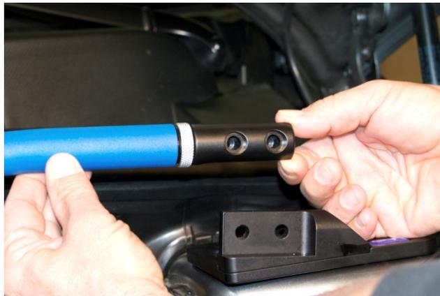
4. On opposite side of vehicle, adjust billet-end clevis holes to match-up to base plate hose. In order to slide clevis onto base plate, rotate bar as necessary. **NOTE:** Adjust so that an equal amount of thread is exposed on each side of tie-bar.
