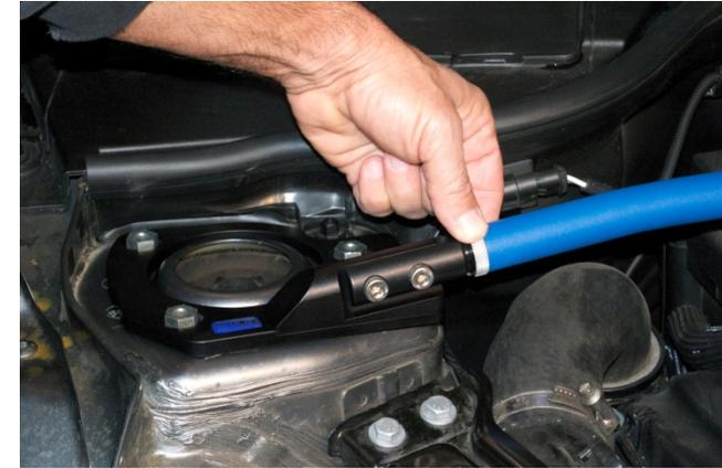
6. Now hand tighten locking collar on each side of tie-bar. Installation is complete.
