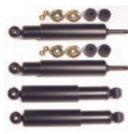
The purpose of a shock absorber is to keep the tire in contact with the road in bad conditions. If your car keeps hopping or moving after you hit a bump in the road, then you need new shocks. The "KYB" brand
