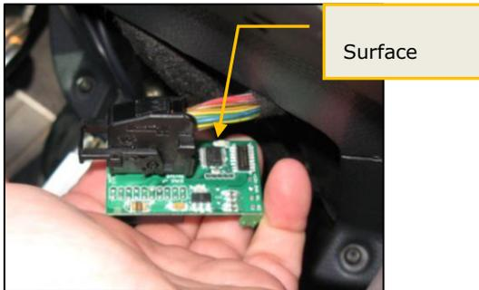
Once the original connector is removed, it can be connected onto the MINI circuit. The connector can be fitted many ways, but only one is correct! You must have the connectors wire bundle exiting from the side that has the piezo and 4 pin accessory header, and you must have all 18 pins connected.
