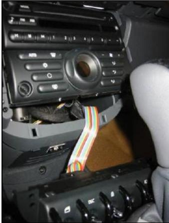
This picture from Bill shows the MINI circuit pushed in behind where the toggle switch panel normally fits, with the harness from it going to the toggle switch panel (the downtubes are still removed)
