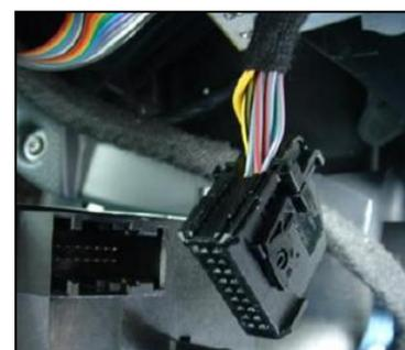
I find it easier to reach the connector from the left side of the car (driver side in USA). Be careful not to reach very high into the car, where this is a similar feeling connector to the a/c controls!
