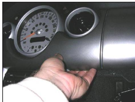
Remove the T20 Torx screw that secures lower passenger side edge of the dash center fascia near the airbag panel (not present on all MINIS):
