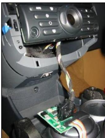
This picture from Bill shows the downtubes removed, the toggle switch panel removed, and the original toggle switch panel connector plugged into the MINI circuit.
