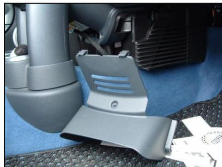
For 2002-2004 Minis, this panel is removed for the "blind" install - it is held by one Torx™ screw (T20) and some clips. Here the trim piece is removed:
