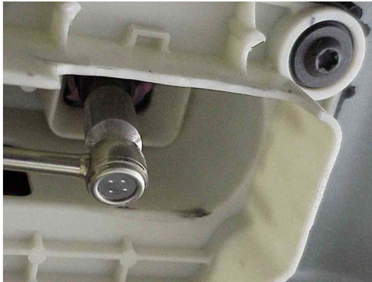
7. COOPER AND COOPER S - In order to accept a modified bottom cover, some of the tabs and structures need to be ground away.
