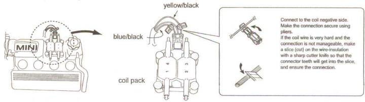
5 Connect the Quick Connector Bs to the Plasma Booster blue colored-wires using the Crimp tool.
