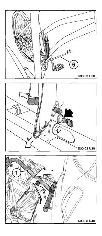
27. Secure lower section of bike frame to rack using nylon straps routed around bike frame and through Tie-Down Strap Arm (6) loops.
