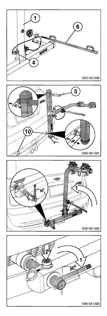
10. Install Tie-Down Strap Arm (6) onto Pivot Arm (1) as illustrated.
