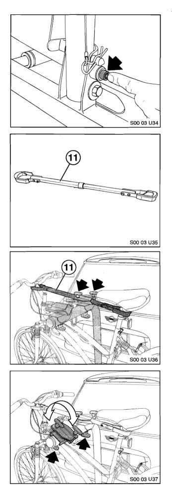
21. To lock Pivot Arm in place push security lock inward as illustrated.
