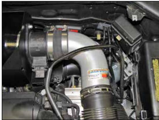
13. Install the K&N® intake tube into the factory intake hose and then into the hose at the mass air sensor. Secure the intake tube with the factory and provided hose clamp.
