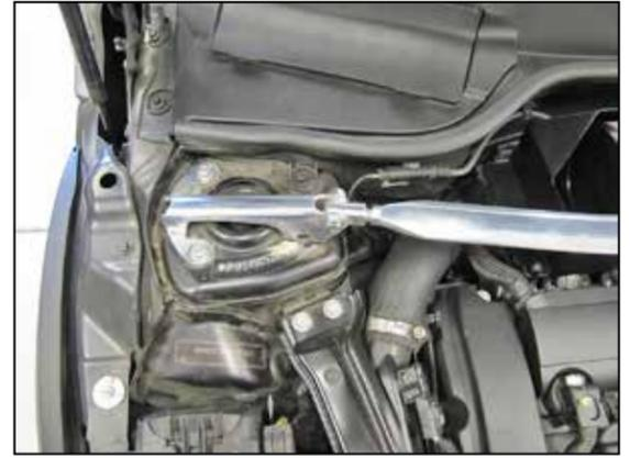
15. Reinstall the strut tower brace and secure with the factory hardware.
