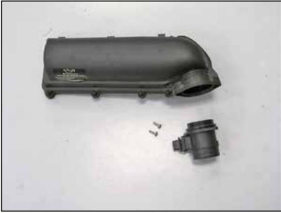
7. Remove the two screws securing the mass air sensor housing to the air filter housing and then remove the mass air sensor as shown.
