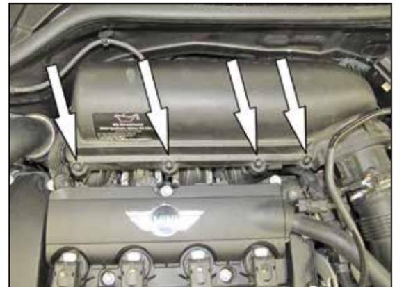
5. Loosen the four screws securing the upper air box housing to the lower housing.
