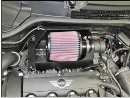
11. Install the K&N® heat shield assembly and secure with the two factory air box screws from the previous step.
