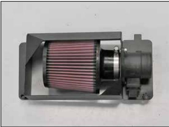
9. Install the K&N® air filter onto the mass air sensor and secure with the provided hose clamp.
