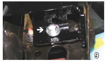
Hold the baseplate up in place and start the 8MM-1.25 x 50MM hex bolt with lock and two flat washers into existing hole. Do to both sides of the vehicle. Clamp the baseplate in place.
