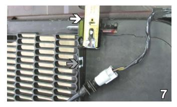
7. Located on both sides behind the grill, there is a temperature sensor that will need to be moved. Trim 1 1/8" from the top to remove the notch holding the sensor, cut and remove the webbing with it, and replace the sensor in another notch we will cut out a little further down (gray arrow).
