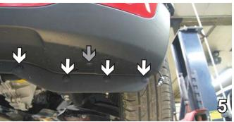
5. Remove four pushpins from the edge of the bottom of the fascia on both sides. There is also a torques 25T bolt (gray arrow) to be removed from both sides using a torques wrench. There are three other pushpins in the center, remove them. Eyebolts need to be removed from the fascia to remove the fascia. Pull the fascia forward, disconnect side running and fog lights. Set aside for later reinstallation.
