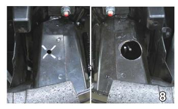
8. Using an existing hole on top of the metal bumper drill a hole using a 1 1/4" hole saw to cut opening for front end to install nut plates. Do this on both sides.
