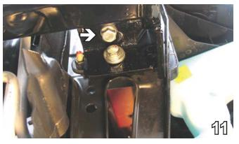
11. Insert 3/8-16 x 1 1/4" bolts with Loctite, 3/8" lock washers and 3/8" nut plates into the drilled holes on the bottom. Do this on both sides.
