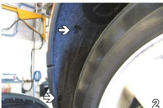
Forward the front tire, there are two pushpins that need to be removed. Do this to both sides. Use a flat screwdriver and set aside for later reinstallation.
