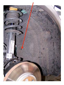
After removing the fender liners use needle nose plyers to pinch and remove the grey colored clips holding the fender flares in place.
