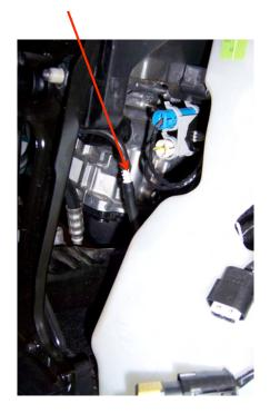
With a friend test the spray pattern for accurate spray pattern. If adjustments need o be made you can use a small screwdriver to pivot the nozzle up and down to adjust pattern. To see the proper spray pattern view the <u>video</u> on our website by clicking on this <u>link</u>.
