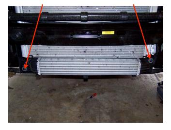
Remove 2, Torx bit screws that hold the intercooler in place
