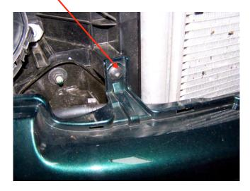
Remove Lighting plugs and temp plug to remove bumper cover
