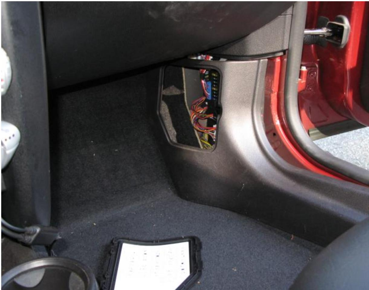
The panel is held on with 5-8 little white snap-fit connectors. Don't worry if some stay attached to the body shell, they are easily removed by hand or by using some pliers and just slide back into slots on the plastic panel. Work the panel free and set it aside.
