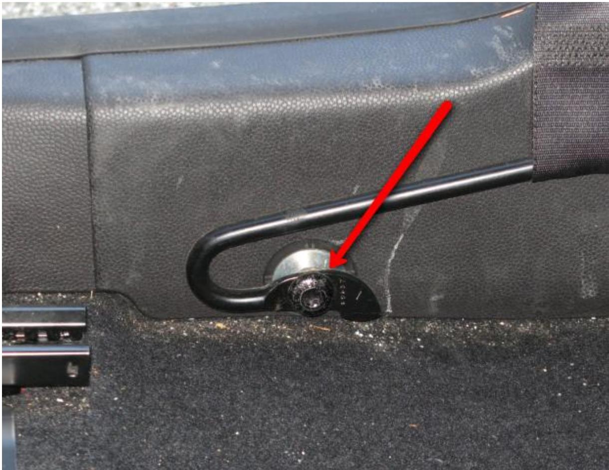
Raise the seat to its highest position and slide it to the rear to gain some access. Now pull the panel toward the center of the car.
