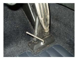
4. Lift up on the accelerator pedal module to access the connector on the back side.
