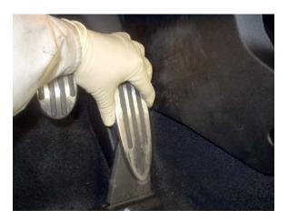
5. Flip the accelerator module on its side to expose the electrical connector. There are latches that need to be 'released' in order for the connector to unplug. While holding the module with one hand, squeeze the connector on the sides with your other hand (squeezing the latches) as you pull it free. It's a little tight, but it will come free.
