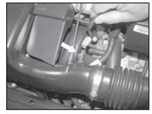
2. Remove the stock crank case vent hose from the cam cover as shown.
