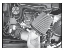
13. Slide the intake tube assembly into the silicone stepped hose & adjust for best fit & clearance as shown.
