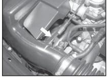
3. Using a pair of side cutters cut the factory hose clamps on the stock intake tube at the throttle body and at the air cleaner assembly as shown.
