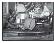
11. Secure the silicone stepped hose & hose clamps onto the throttle body as shown.
