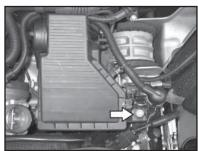
8. Models from 2005: Remove the single bolt that secure the air cleaner assembly as shown.
