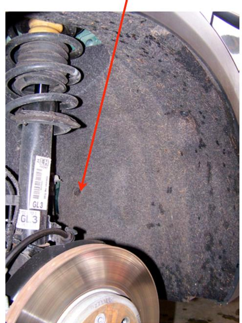
After removing the fender liners use needle nose pliers to pinch and remove the grey colored clips holding the fender flares in place.
