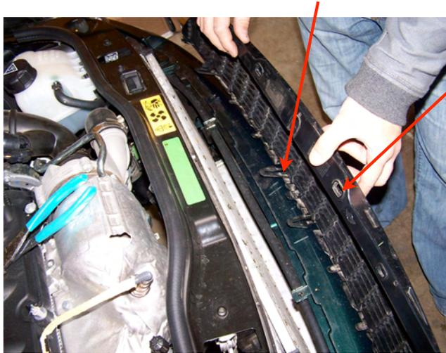
Remove the screws and clips in the lower bumper
