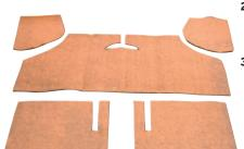
2. Bulkhead fire wall sound deadening piece for MK1/2 and vans etc. ......24A280
