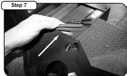
Place the trim seal along the edge of the housing. Position the new housing into the engine bay.
