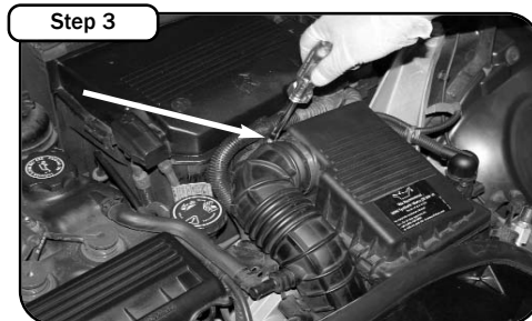
Remove the hose clamp connecting the air duct to the air box. Use a screwdriver to remove the clamp.
