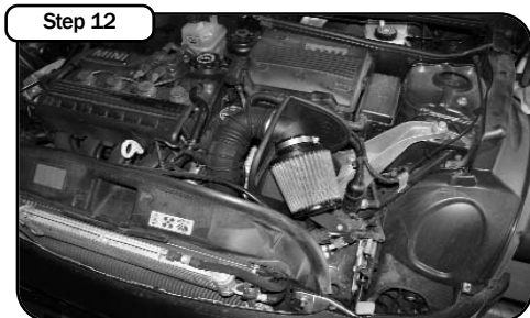
Your installation is now complete. Make sure you tighten all clamps and check all electrical connections. Re check periodically.
