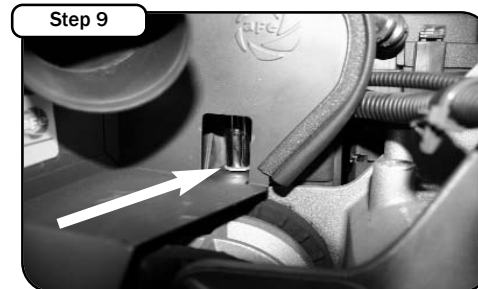
With 10mm socket w/ extension, Re install the rear air box bolt removed in step 5.
