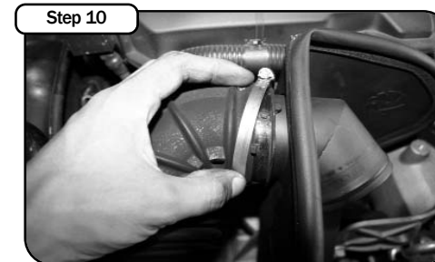
Place the new #044 clamp on the intake duct and tighten assembly to the housing inlet.
