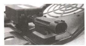
To reinstall the new blower motor, slide the connector back into the white plastic base.
