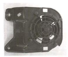
Put the metal housing and the blower motor on top of each other. Align the four screw holes. Slowly screw the housing into the blower motor.
