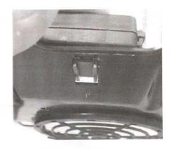
Slide the control unit bracket into the rectangle hole of the metal housing.
