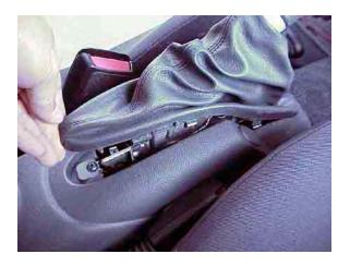
8. Once the boot and grip assembly is removed, turn the boot inside out to expose the part of the grip covered by the boot. You will note the grip is secured to the boot with a plastic cable tie. Cut the cable tie and this will release the handbrake grip.
