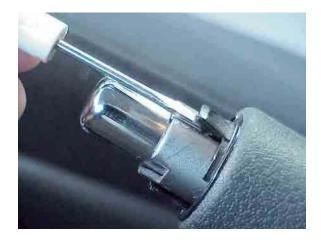
4. Insert a small screwdriver between the boot and the Handbrake Console.
