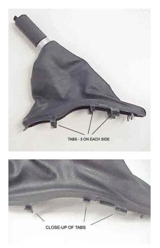
7. Gently lift the boot assembly from the Rear and lift up and out over the handbrake handle.
