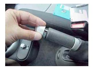
3. Using a small screwdriver, gently lift the tab until it clears the slot. Pull on the Grip and slide towards the Release Button.
