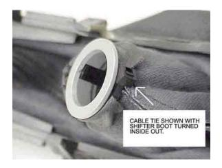
9. Insert the new grip and secure with a similar cable tie. Assemble in reverse as shown above.
