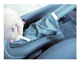
5. Gently pull the screwdriver handle away from the handbrake while pushing down on the rim of the boot so the tip forces the boot rim away from the console.
