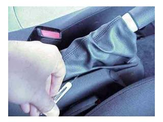
6. Repeat step 5 until all tabs are released from the console. There are 3 tabs on each side of
