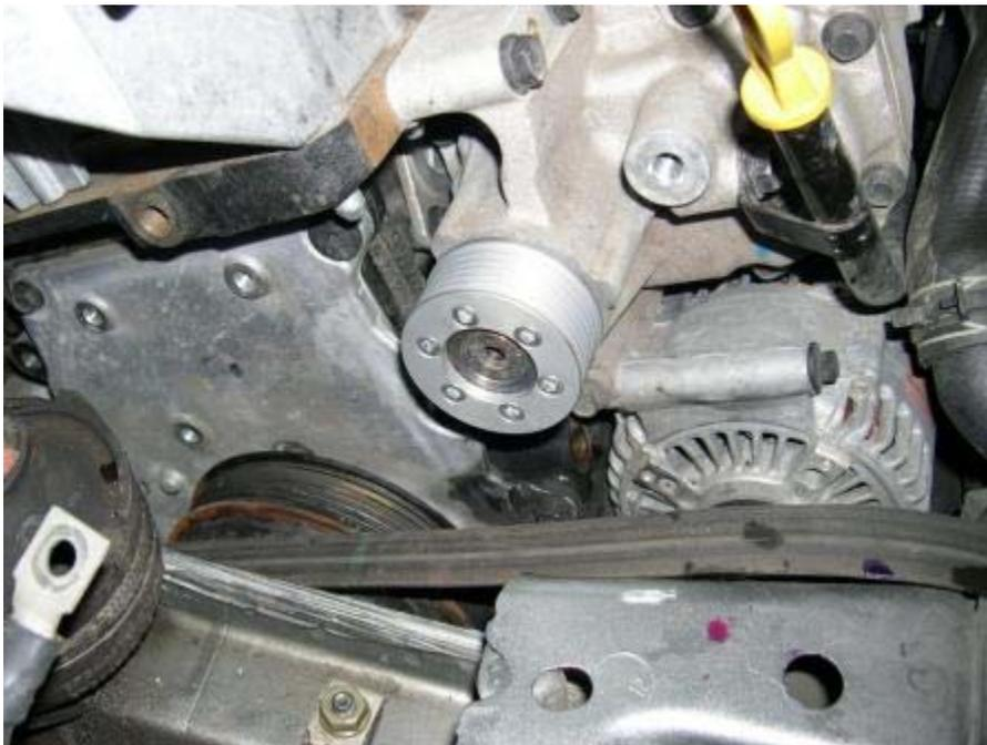
19. Reinstall the tensioner with the two 16mm and two 10mm bolts. After you have it installed,
