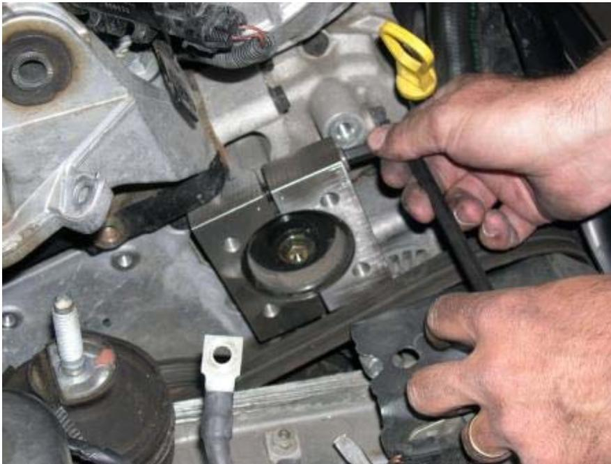
Now install the crow's foot puller onto the removal tool.
