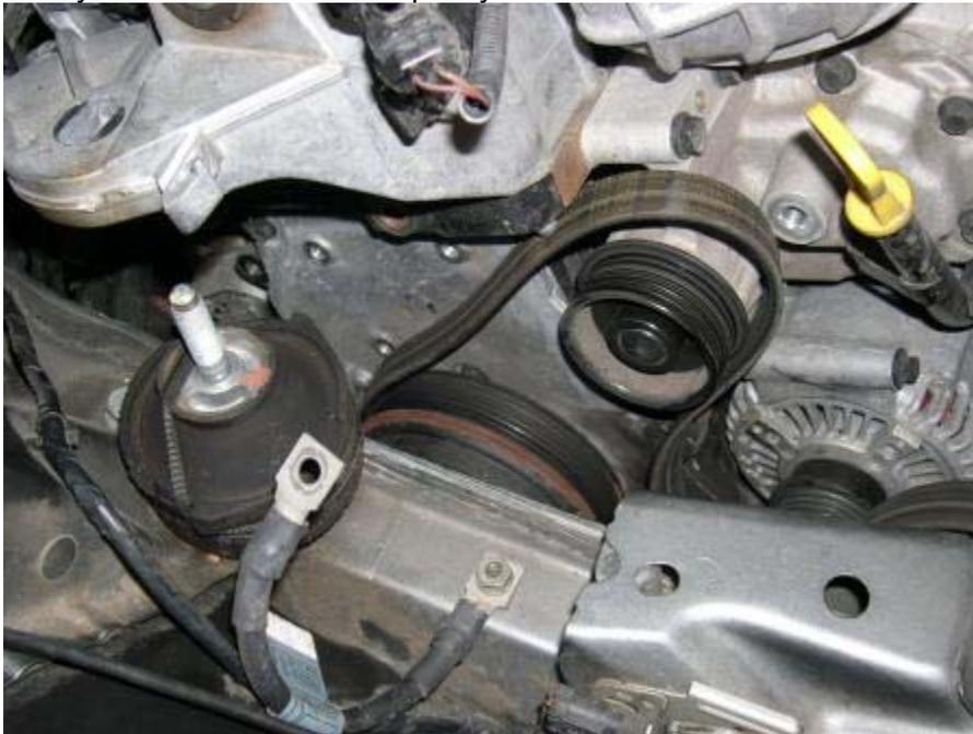
17. Install the pulley removal tool. Start by taking the plastic center cap out of the s/c shaft. It helps to get the lip out slightly with the blade of a standard screwdriver, then it will just thread right out like a bolt by hand.
