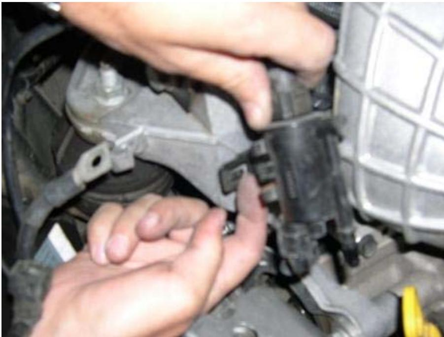
11. There are three hoses attached to the vibration damper bracket. These just pop out of their respective holders (MY '02 - '04). **For Model Year 2005-2006, skip to step 13a.**
