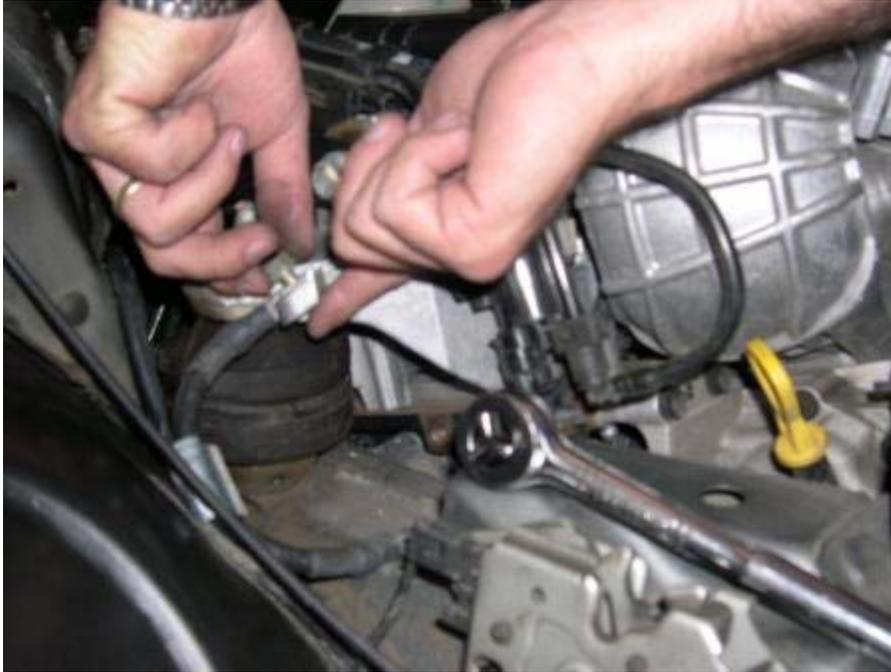
10. I slide the regulator off its bracket to gain more room for the tensioner tool, but you don't really have to. Remove the quick disconnect fittings and use a screwdriver to push the tab on the bracket in slightly and slide it off toward you.
