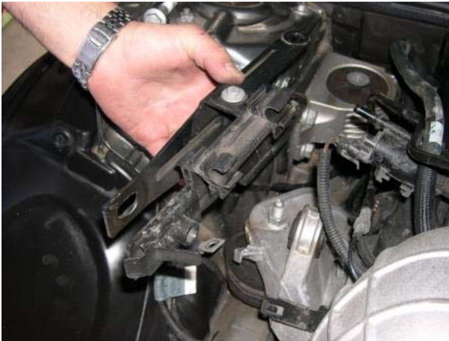
13. Using the 18mm wrench or deep socket, remove the passenger side motor mount nut (MY '02 - '04).
