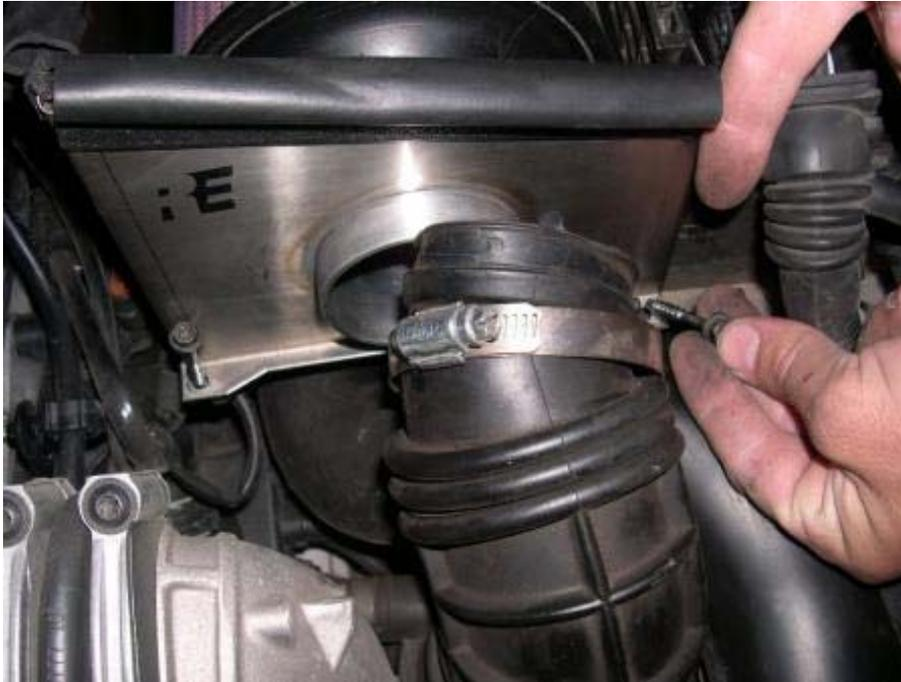
Remove the intake or the panel filter and airbox top (depending on what you have).
