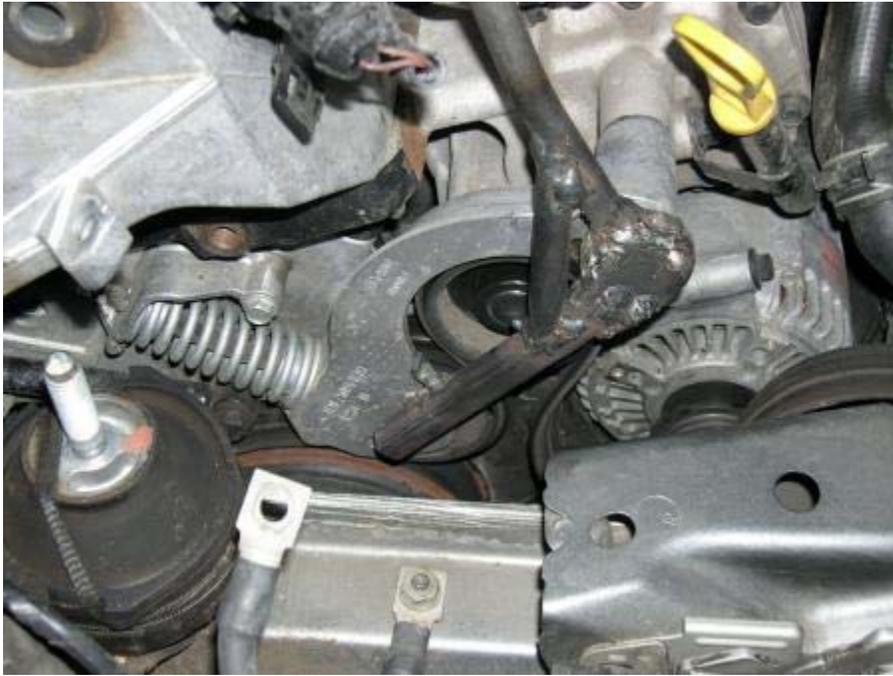
16. Remove the belt tensioner. There are four bolts, two 10mm and two 16mm.
