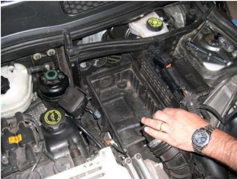
3. Remove the ECU and lower airbox half. Remove the ECU cover (it just has two tabs on each side that squeeze together and pull off), then remove each of the two plugs. These are a little tricky - they have tabs on the end of the plug that pull away from the plug which forces the plug up and off. It's easiest to use a small screwdriver very carefully to pull these tabs away from the plug.
