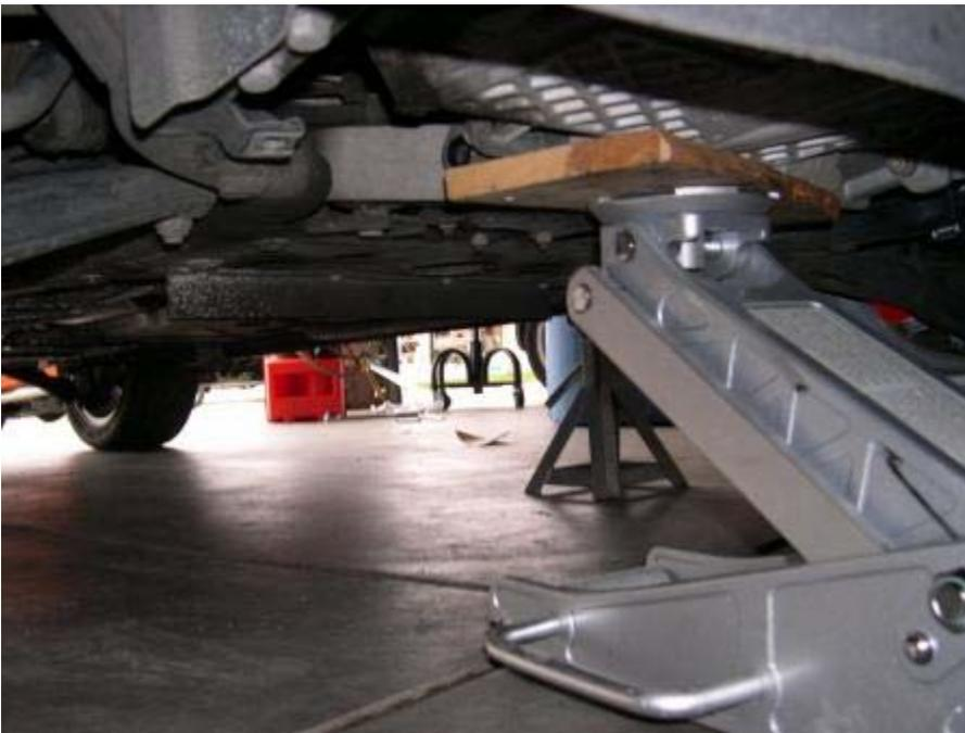
7. Remove the driver side 16mm motor mount bolt. It helps to wiggle as you are pulling it out, and jacking slightly may help as well. It is a little bit of an art, but once you get the hang of it, it is pretty easy (and it is the same thing threading it back in - you get good at it by just wiggling and jacking the motor at the same time).
