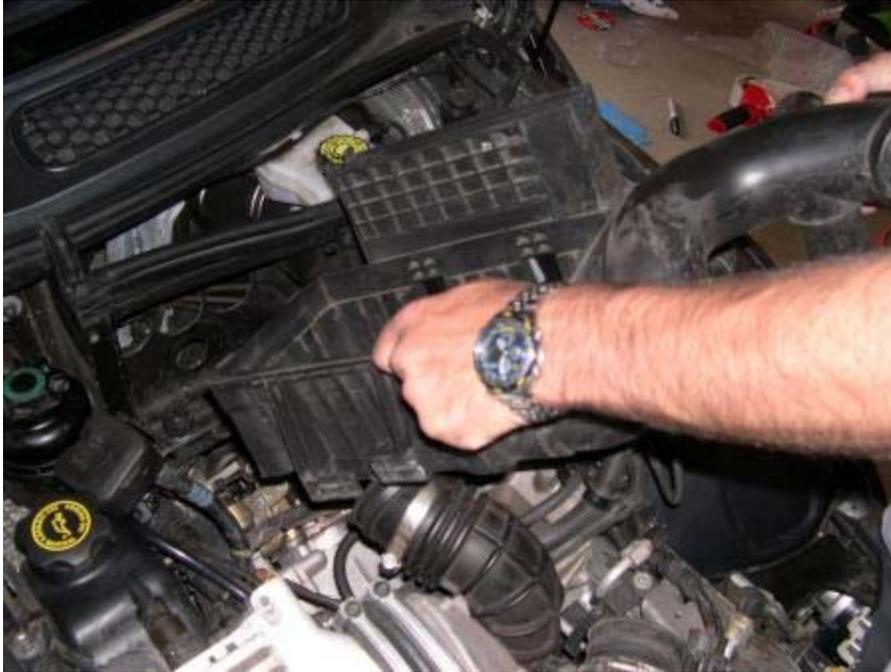
Here's what it looks like with the box removed. Note the two small rubber mounting bolts at the bottom rear of the partition. The box is molded on the underside to fit into these mounts, which is why you had to pull toward the front of the car before you pulled up and out.
