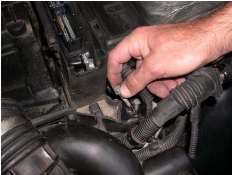
Now remove the clamp on the snorkle to the airbox. You will either use a standard screwdriver if you have replaced the clamp, or the factory removal tool if you still have the stock clamp (you can also remove the stock clamp with a small screwdriver and replace it with the screwdriver and small
