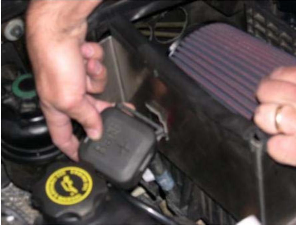
Remove the clamp at the intake boot.
