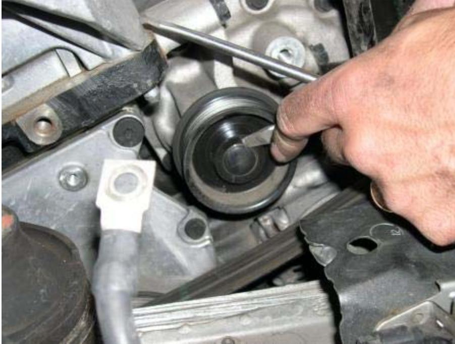
Install a 13mm bolt into the center of the shaft. Slide the two halves of the removal tool over the pulley and tighten the allens. Photo below may show a different shaped pulley removal tool.
