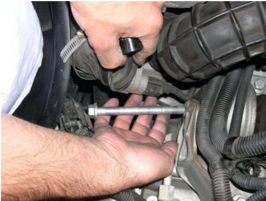
8. Remove the 10mm clamp bolt holding the wiring loom and radiator hose to the intake manifold.
