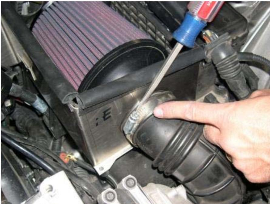
Remove the two #25 torx bolts at the base of the intake heat shield (or if it is the stock box, these same two bolts hold the top of the airbox in place).
