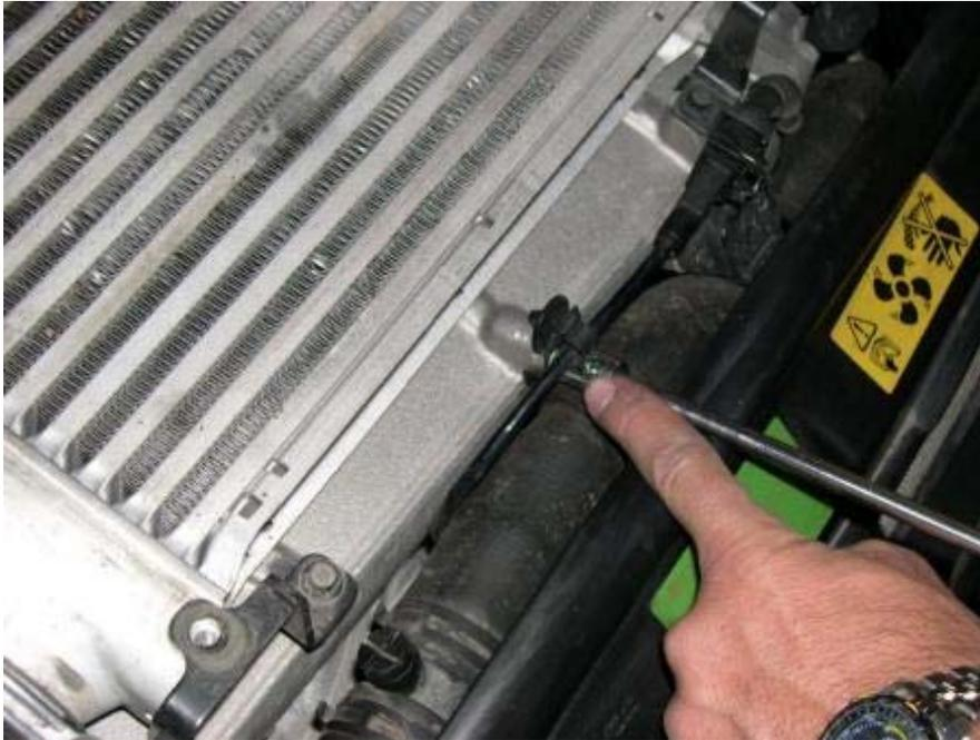
9. Remove the 13mm ground bolt from the passenger side motor mount.
