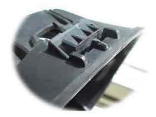
This is the clip at the 3 o'clock position, notice more structures limiting access to the clip.
