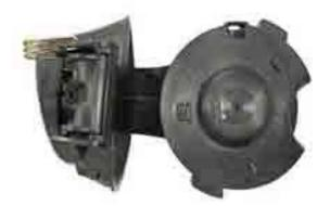
3. There are 3 clips holding the fuel filler cap assembly in place which need to be released <u>without removing the filler assembly</u>. Using a dull flat tool such as a plastic putty knife, carefully release the clips by sliding the tool inbetween the bodywork and the filler cap assembly. Location of the clips are evident by the indentation within the cap assembly. (They are located at the 1 o'clock, 3 o'clock and 7 o'clock positions.)
