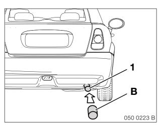
Connect the accessory tailpipe trim **B** onto the tailpipe (1).
