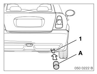
Connect the accessory tailpipe trim **A** onto the shortened tailpipe (2).
