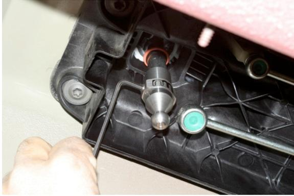
7. Install NM adapter onto end of shift lever with set screws facing front to back. Tighten using 3mm Hex Key wrench. With shift lever fully seated into adapter set screws should be almost flush with adapter body.
