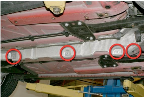
4. Remove forward tunnel heat shield. There are 3 tin nuts and 1 plastic nut on each side.
