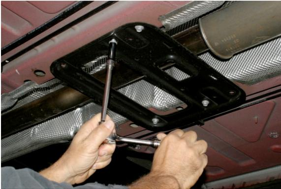
2. Remove exhaust tunnel cross-brace, (4) 10MM Hex Bolts.
