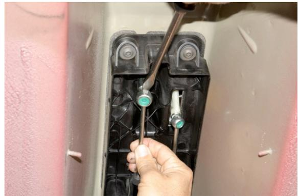
6. Pull down on the cable while prying opposite side with large screwdriver to disconnect from shifter.
