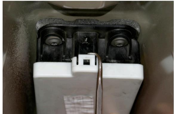
5. While pulling down on bottom shifter box cover with your fingers, carefully pry outward locking tab to unhook, do the same to the rest of the tabs around shifter box.
