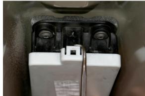
While pulling down on bottom shifter box cover with your fingers, carefully pry outward locking tab to unhook, do the same to the rest of the tabs around shifter box.
