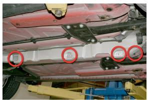
Remove forward tunnel heat shield. There are 3 tin nuts and 1 plastic nut on each side.
