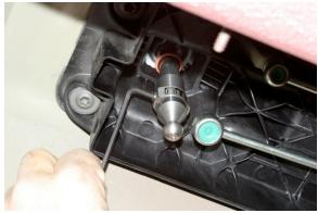
Install NM adapter onto end of shift lever with set screws facing front to back. Tighten using 3mm Hex Key wrench. With shift lever fully seated into adapter set screws should be almost flush with adapter body.
