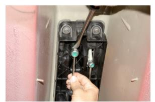
Pull down on the cable while prying opposite side with large screwdriver to disconnect from shifter.
