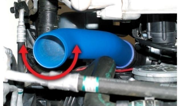
11. Rotate pipe for correct position, bottom opening of pipe should be parallel to the ground and there should be no interference with any other vehicle components.
