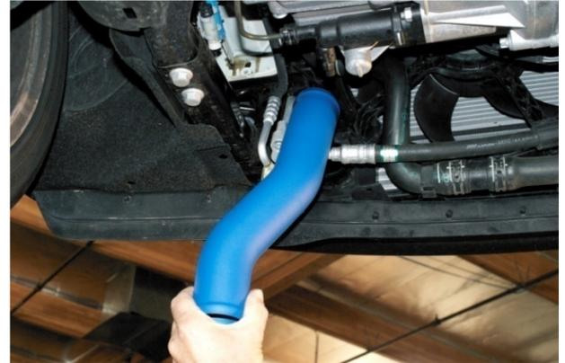
10. From underneath vehicle install aluminum pipe (longer straight section goes up). Use WD-40 on pipe ends for easier fitment.
