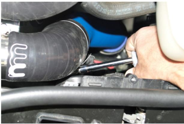
14. Before tightening upper aluminum pipe hose clamp, it must be rotated toward front of vehicle so not to interfere with coolant hose. Once again remove coolant reservoir tank and set aside to ease access to clamp for tightening. Now tighten.
