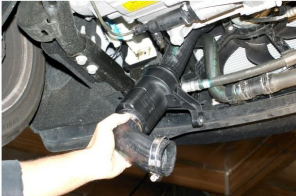
6. Loosen clamp (7mm hex) at lower pressure hose to intercooler; now remove hose and muffler downward from vehicle.
