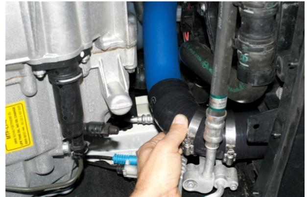
12. Install 90° silicone hose with supplied #40 hose clamps. **NOTE:** Slightly longer straight section on hose goes toward intercooler.
