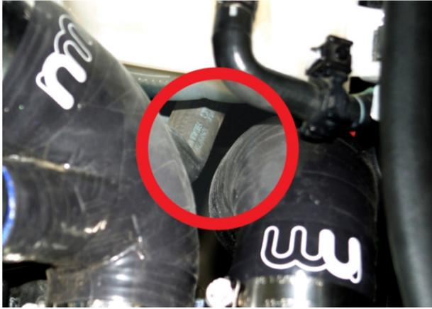
8. Rotate custom silicone hose so that there is about a 3/8" clearance between it and the coolant hose. Then tighten hose clamp (8mm hex).
