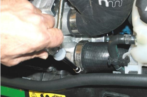
3. Loosen turbo discharge hose clamp (7mm hex) and disconnect hose from turbocharger.
