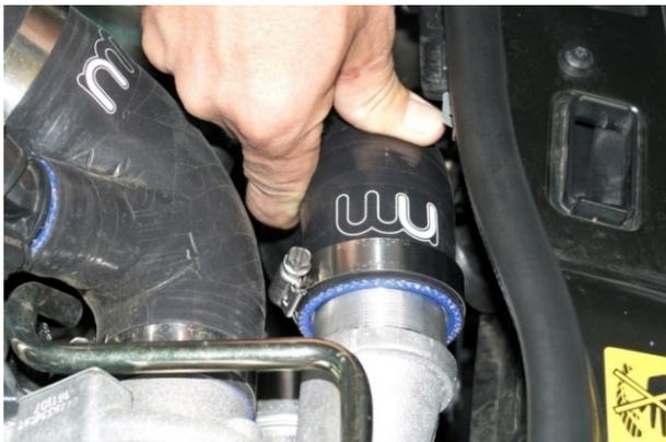
7. Attach custom silicone hose with supplied #28 hose clamp to turbo; do not tighten at this time. Temporarily remount coolant tank. **NOTE:** Coolant hose runs above lower pin mount.
