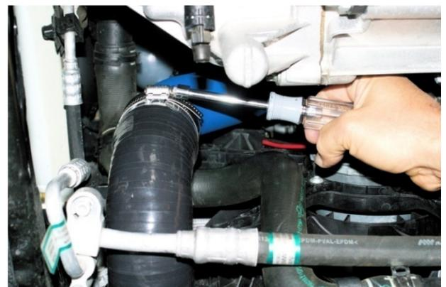
13. Now tighten 90° silicone hose clamps (7mm hex). Double-check pipe for proper clearances from top to bottom.
