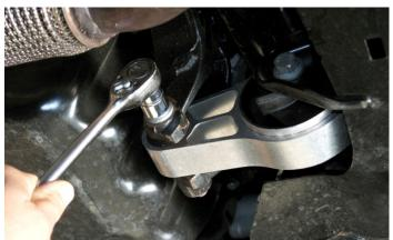
2. Underneath the vehicle: Unbolt the [2] 16mm hex bolts to remove the engine torque arm.
