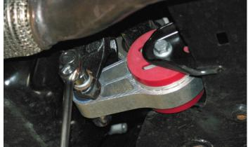
4. Reinstall torque arm and torque bolts to 80 foot/pounds or 108 nm. Double check installation.
