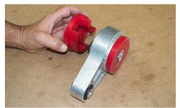
Install NM Engine Torque Arm Insert into each side of OE torque arm. NOTE: Red urethane used for picture clarity.
