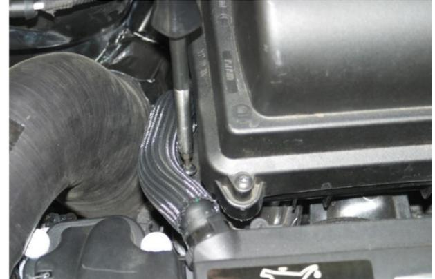
6. Remove T25 TORX screw located on passenger side of air filter box and lift off. **NOTE:** There are [3] pin mounts that are pushed into rubber grommet mounts on intake manifold, so effort may be required to lift air filter box off of mounts.
