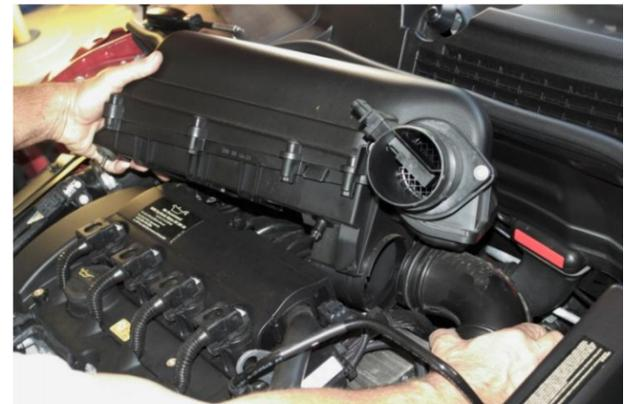
7. Locate fresh air pipe that is attached to air filter box. Disconnect fresh air pipe by rotating the 90° connection counter clockwise and pulling pipe away from air filter box. Remove air filter box from vehicle.
