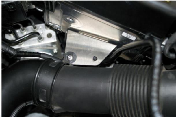
13. Attach brake booster line holder to forward mounting hole in bracket. Secure fresh air pipe to rearward mounting hole using supplied M6 x 10mm button head bolt. [4mm hex key wrench]
