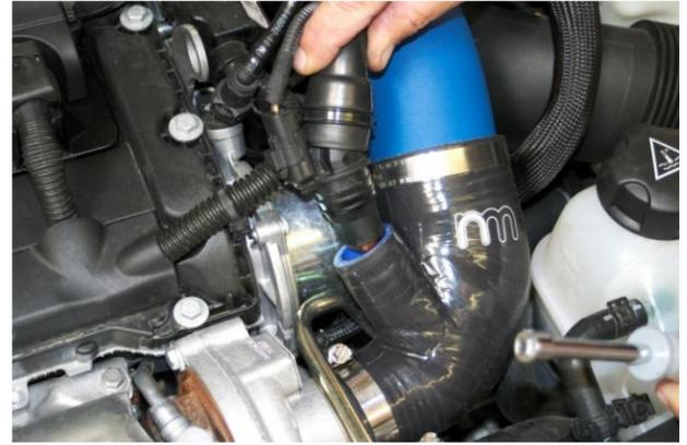
17. Install valve cover breather into silicone turbo inlet hose.
