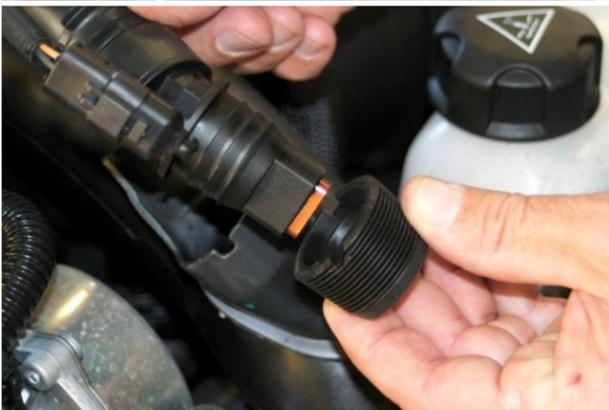
1. **JCW Only:** Cut wire tie at valve cover breather hose to OE turbo inlet hose. Pull out breather hose and remove rubber collar. Then proceed to step #3.
