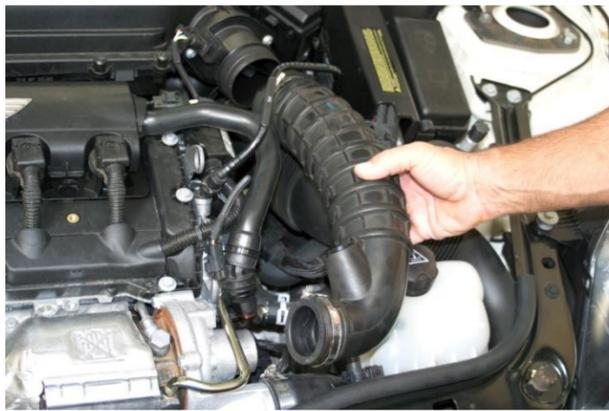
3. Remove OE turbo inlet hose from MAF sensor. Use screwdriver to loosen clamp at turbo inlet and at MAF sensor.
