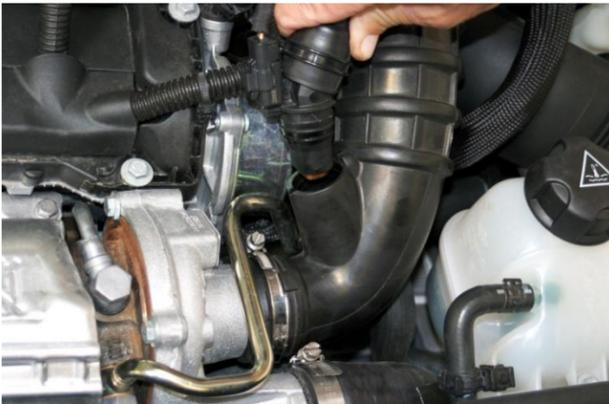
2. **S MODELS ONLY:** Pull out valve cover breather hose from OE turbo inlet hose.
