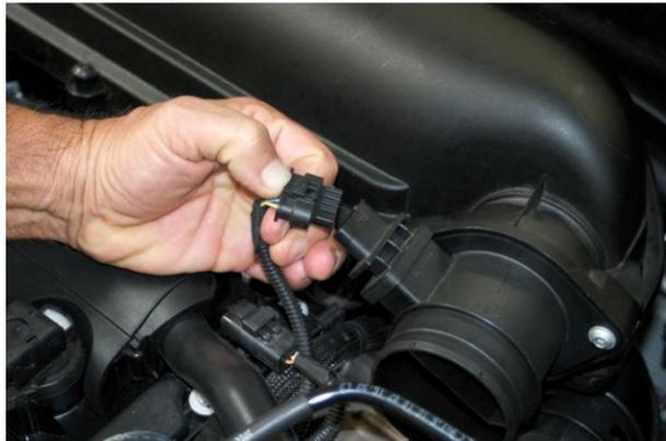
4. Disconnect electrical connector from Mass Airflow Sensor (MAF).
