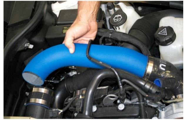
16. Loosely install supplied #44 clamps onto both silicone hose ends, then install aluminum intake pipe into silicone turbo inlet hose **first** and then into MAF sensor hose. Adjust as necessary for clearance, paying close attention to clearance of silicone turbo inlet hose and coolant reservoir bottle. Tighten all clamps, use caution **NOT** to over tighten on Carbon Fiber Tube if being used. **NOTE:** Do not forget to tighten #28 hose clamp from Step 14.
