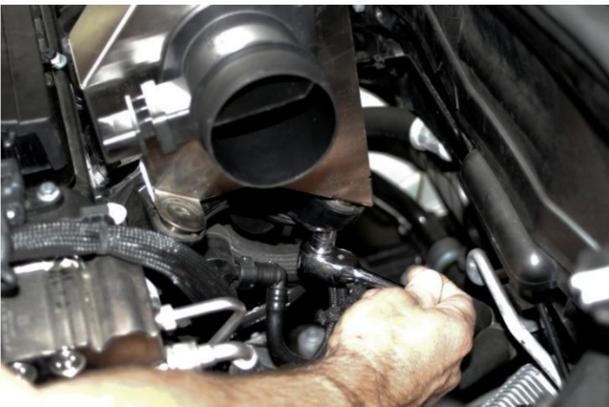
11. Install NM filter assembly unit onto factory air filter box mounts. **NOTE:** Make sure rubber grommets are still in place and not attached to bottom of the OE air filter box. From bottom side of mounts, install and tighten using supplied M8 washers and M8 lock nuts. [13mm socket and wrench]
