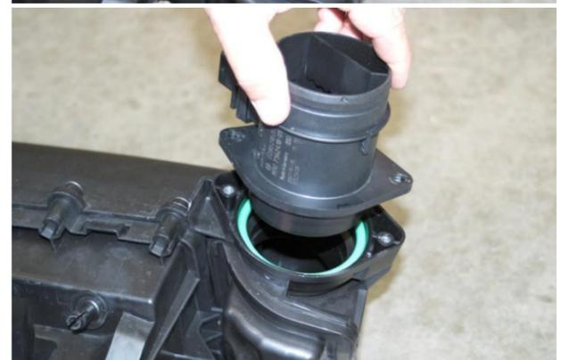
8. Remove MAF sensor from air filter box by removing [2] T30 TORX screws.
