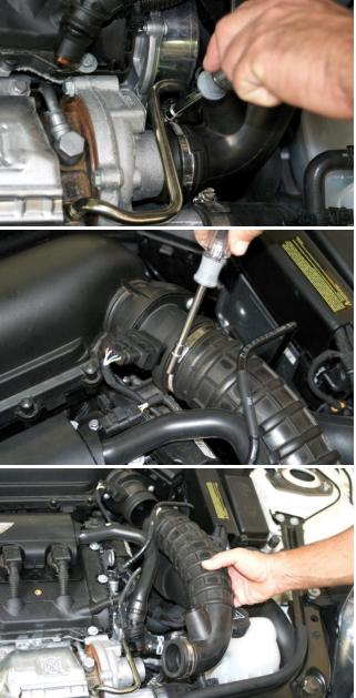
Remove OE turbo inlet hose from MAF sensor. Use 3 screwdriver to loosen clamp at turbo inlet and at MAF sensor.
