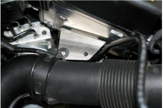
Attach brake booster line holder to forward mounting hole in bracket. Secure fresh air pipe to rearward mounting hole using supplied M6 x 10mm button head bolt. [4mm hex key wrench]
