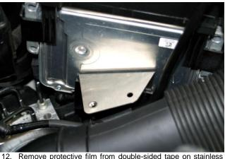
Remove protective film from double-sided tape on stainless steel fresh air hose bracket. Slide bracket down between ECU and black plastic ECU mount, while keeping double stick tape from touching. With bracket pushed all the way down, press against ECU.
