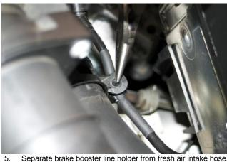
Separate brake booster line holder from fresh air intake hose. Use needle nose pliers to squeeze tabs and then push out holder.
