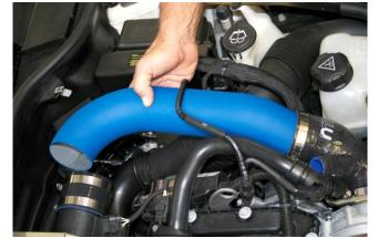
16. Loosely install supplied #44 clamps onto both silicone hose ends, then install aluminum intake pipe into silicone turbo inlet hose <u>first</u> and then into MAF sensor hose. Adjust as necessary for clearance, paying close attention to clearance of silicone turbo inlet hose and coolant reservoir bottle. Tighten all clamps, use caution NOT to over tighten on Carbon Fiber Tube if being used. <u>NOTE</u>: Do not forget to tighten #28 hose clamp from Step 14.
