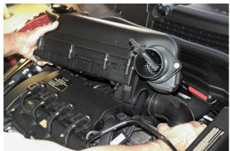
7. Locate fresh air pipe that is attached to air filter box. Disconnect fresh air pipe by rotating the 90° connection counter clockwise and pulling pipe away from air filter box. Remove air filter box from vehicle.
