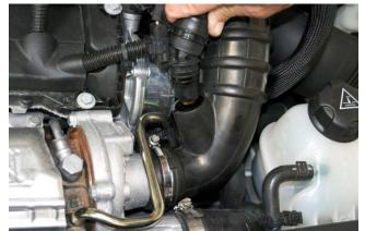
S MODELS ONLY: Pull out valve cover breather hose from 2. OE turbo inlet hose.
