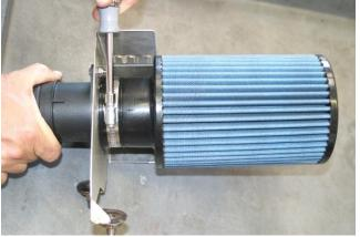
Using degreaser or contact cleaner and shop rag, clean inner mounting flange of NM filter. Install and tighten filter onto MAF sensor. Position NM logo on end of filter for proper reading orientation.
