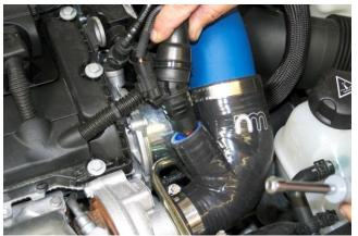
17. Install valve cover breather into silicone turbo inlet hose.
