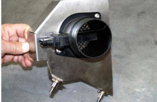
Install MAF sensor to NM stainless steel intake pipe bracket using supplied M6 x 16mm button head bolts and M6 nuts. [4mm hex key wrench / 10mm socket or wrench]
