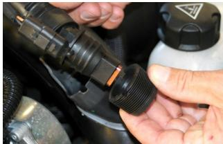
JCW Only: Cut wire tie at valve cover breather hose to OE 1. turbo inlet hose. Pull out breather hose and remove rubber collar. Then proceed to step #3.
