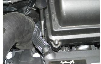
Remove T25 TORX screw located on passenger side of air filter box and lift off. NOTE: There are [3] pin mounts that are pushed into rubber grommet mounts on intake manifold, so effort may be required to lift air filter box off of mounts.
