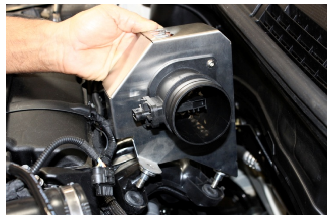
7. Install MAF sensor to NM stainless steel intake pipe bracket using supplied M6 x 16mm button head bolts and M6 nuts. [4mm hex key wrench / 10mm socket or wrench]
