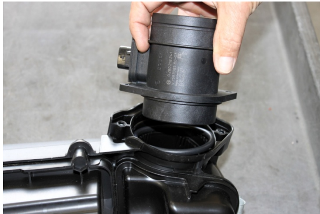
6. Remove MAF sensor from air filter box by removing [2] T30 TORX screws.
