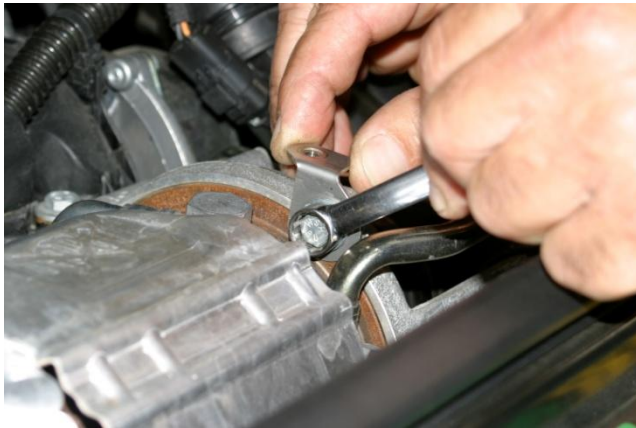
2. Mount supplied SS Support Bracket to turbo housing using original bolt.
