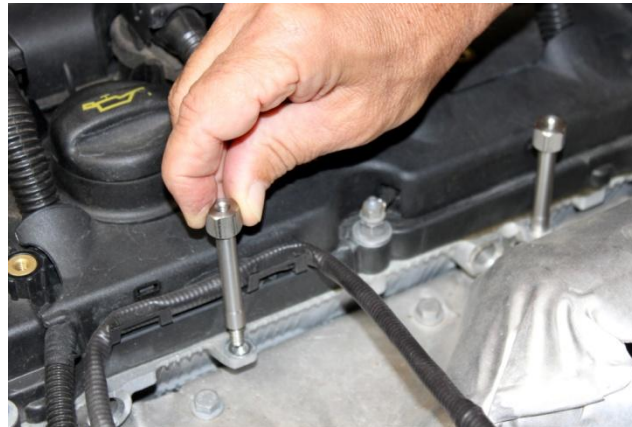
4. Install Hex Stand-offs with 6MM SS washers (washers not shown) into threaded ears on cylinder head.
