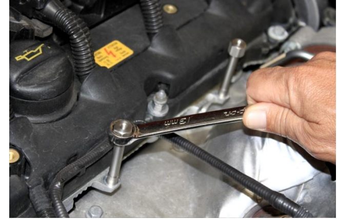
5. Tighten using a 13mm wrench. NOTE: Torque to 10 ft-lbs.
