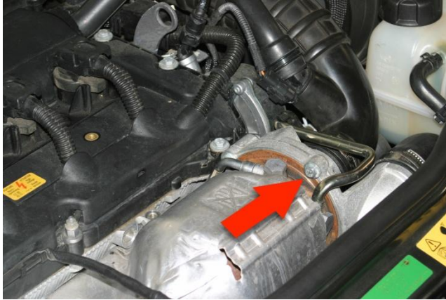
1. Using a 10mm wrench, remove turbo housing bolt.
