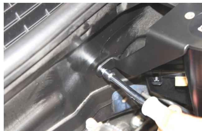
9. Align Catch Tank in vertical position and then using self tapping screw fix Tank bracket to plastic firewall. **Note:** Do not over tighten screw into plastic firewall.
