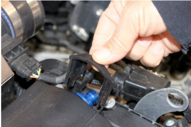
13. Lightly oil "O" rings on supplied billet fitting and install into breather port then reinstall factory retaining clip.
