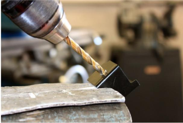
6. Enlarge bracket mount hole using 1/4" drill bit.
