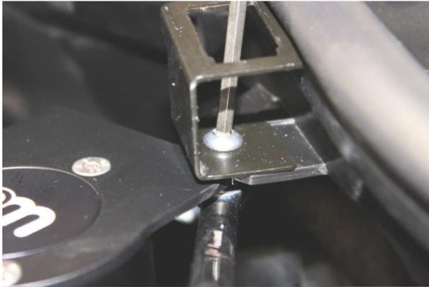
7. Using M6x16mm Button Head screw with washer and lock nut, install in order; switch bracket, plastic mounting tab then Catch Tank bracket on bottom then washer and lock nut. Proceed to step #9.
