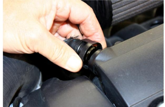
10. Disconnect breather hose at back left side of valve cover by squeezing locking collar. Lightly oil "O" ring on billet plug and install into valve cover port with locking spring clip facing outwards as pictured. Now re-install factory hose onto billet fitting.
