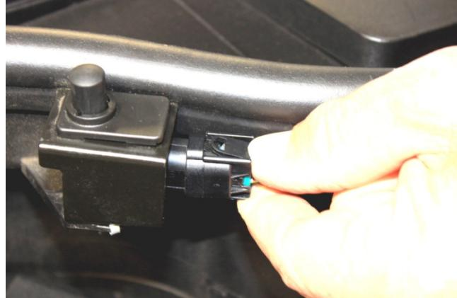
1. **For vehicles with alarm hood switch start here, without switch proceed to step #8.** Remove air intake tube or factory air box for easier access. Disconnect electrical connection by squeezing locking tab and then pull out.
