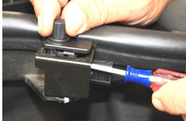
2. Between switch and mounting bracket there is locking tabs on each side, using a small screw driver push in to release.
