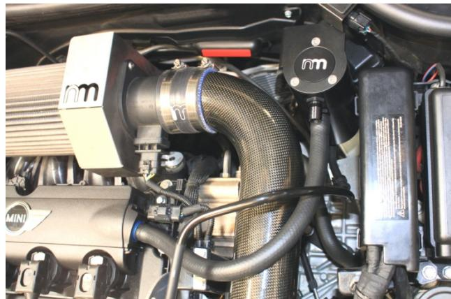
16. Using about 15" of supplied hose install from valve cover to bottom fitting on Catch Tank. Spray WD-40 or equivalent to ease installing hose onto fittings.
