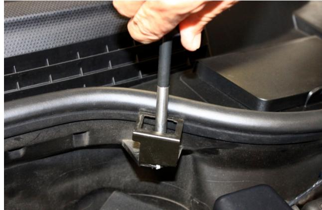
4. Remove bracket mounting screw with a T20 Torx.
