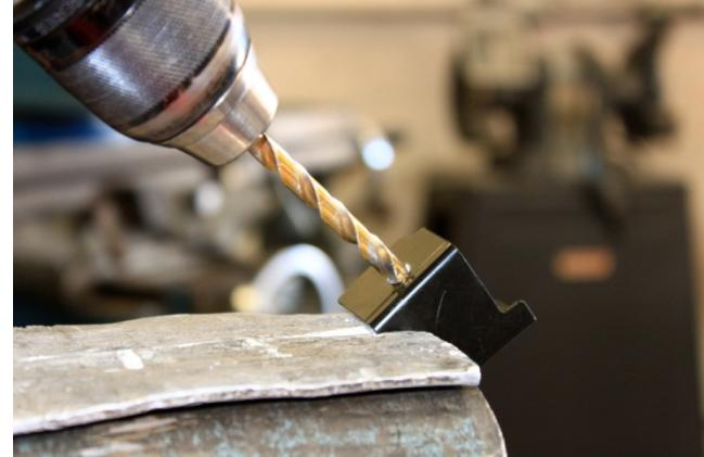
6. Enlarge bracket mount hole using 1/4" drill bit.
