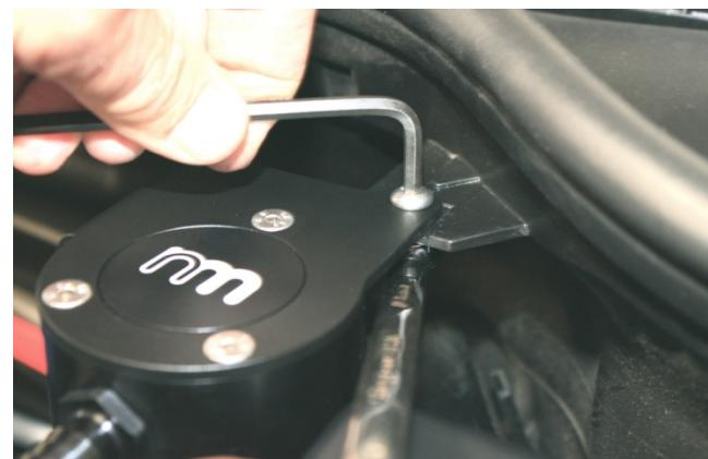
8. **Vehicles without alarm switch start here.** Remove air intake pipe or factory air box for easier access. Using M6x 16mm Button Head screw, washer and lock nut mount Catch Tank to top side of tab on plastic firewall.
