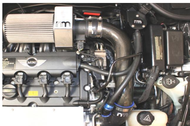
17. Using about 14" of supplied hose install from turbo inlet hose to top fitting on Catch Tank. Spray WD-40 or equivalent to ease installing hose onto fittings.
