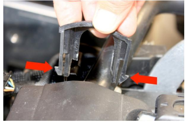
11. Remove right side valve cover breather hose retaining clip by squeezing lock tabs at the bottom, then pull up.
