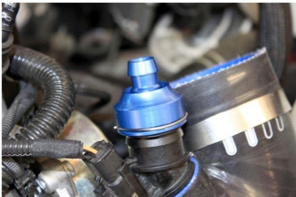
14. Lightly oil "O" ring on billet fitting and install onto turbo air inlet hose.
