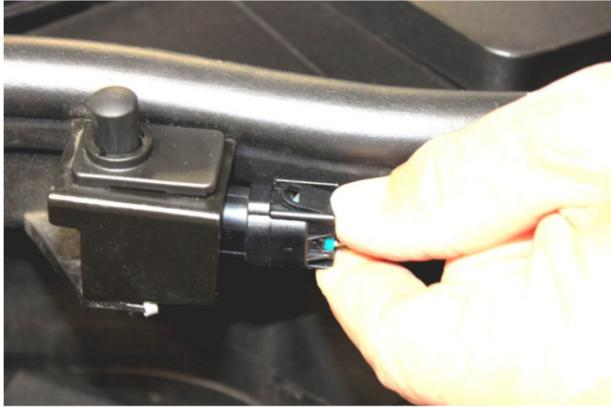
1. **For vehicles with alarm hood switch start here, without switch proceed to step #8.** Remove air intake tube or factory air box for easier access. Disconnect electrical connection by squeezing locking tab and then pull out.
