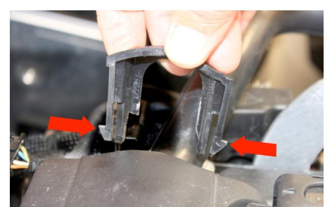
11. Remove right side valve cover breather hose retaining clip by squeezing lock tabs at the bottom, then pull up.
