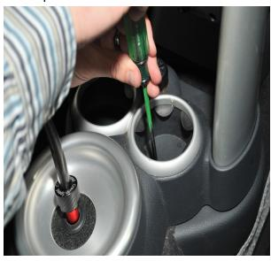
Carefully with a plastic tool or a screwdriver, pinch the middle of the sides of the emergency brake boot. Lift and maneuver the brake boot up, then the entire console can be lifted, but **don't pull!** The power wires to the 12-Volt socket are still in place.
