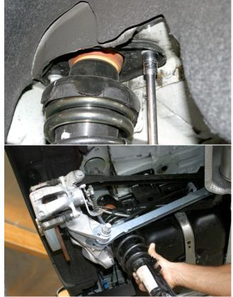
Unbolt and remove [2] upper shock mount bolts using 13mm socket and 18" extension. Remove shock and repeat for other
