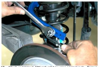
Attach end links to NM anti-roll bar using original nuts. Torque to 30 Nm (22 ft-lbs). See adjustment chart for hole mounting information.
