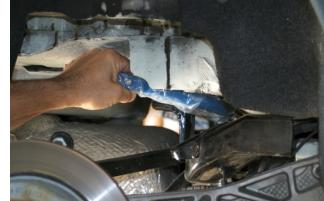
Install NM anti-roll bar in reverse of removal of original bar. HINT: Leave plastic wrap on bar to protect finish of bar during installation thru sub-frame then remove.
