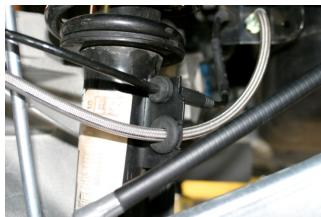
Detach brake line and ABS wire from rear shock absorbers.
