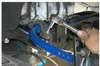
Install billet aluminum clamps over bushings and bolt to subframe using supplied M8 x 25mm bolts. Torque to 33 Nm (25 ff-lbs)
