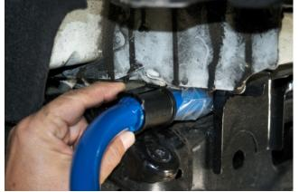
Apply supplied grease to inside of supplied bushings and install on the inside of stop washer on NM anti-roll bar.
