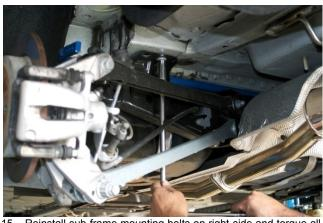
Reinstall sub-frame mounting bolts on right-side and torque all [4] bolts to 100 Nm (74 ft-lbs).
