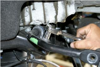
Remove the bushing clamp mounting bolts [2] using a 13mm socket. Remove clamp and bushing. Repeat for other side.
