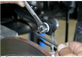
Disconnect end-link from original anti-roll bar by securing stud with 6mm hex key wrench and loosening nut with 16mm wrench. Repeat for other side
