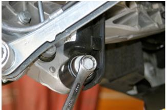
Unbolt and remove lower shock absorber bolt using 18mm wrench
