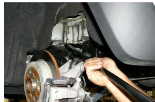
11. Now from left-side of vehicle completely remove original bar.
