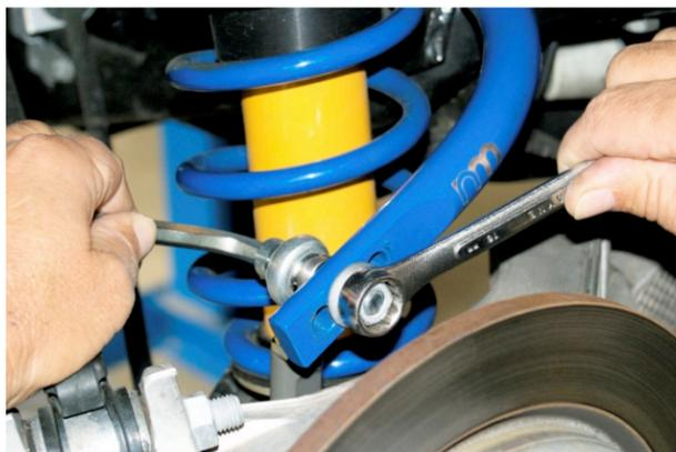
7. Tighten bolt using 8mm hex key wrench and 16mm wrench. Torque to 45 Nm (33 ft. lbs.)
