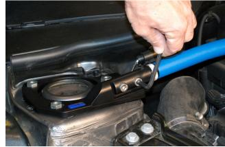
Install and tighten all [4] M8 x 20mm hex socket bolts using a 6mm hex key wrench.
