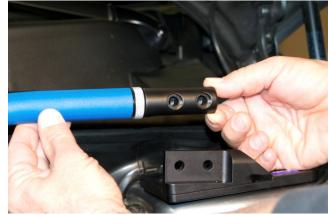
On opposite side of vehicle, adjust billet-end clevis holes to match-up to base plate hose. In order to slide clevis onto base plate, rotate bar as necessary. NOTE: Adjust so that an equal amount of thread is exposed on each side of tie-bar.
