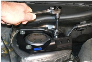
Mount and evenly tighten the NM base plate to strut towers using special long-reach nuts - torque to 34 Nm (25 ft-lbs.). NOTE: Hand thread all nuts to be certain that shoulder of nut centers into NM base plate holes before torquing.
