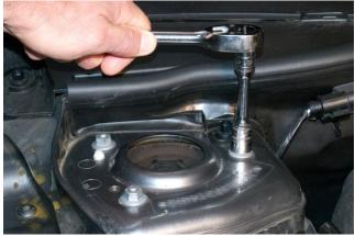
Park MINI on a level surface and remove the [6] 13mm hex nuts (3 on each side) on top of the front strut towers
