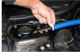
Now hand tighten locking collar on each side of tie-bar. Installation is complete.
