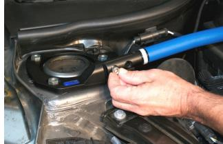
Attach NM aluminum tie-bar to base plate on one side at this time with [1] M8 x 20mm hex socket bolts supplied. Do NOT tighten at this time.
