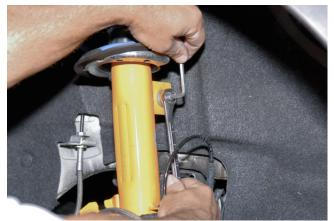
Unbolt end link from strut mount using a 16mm wrench and a 5mm hex key wrench, then remove end link. Repeat for other side.
