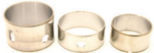
It is also essential to fit cam bearings in any 850cc block being used in competition to prevent seizure of the cam. The block will need to be line-bored by a competent engineering company to enable fitment.
