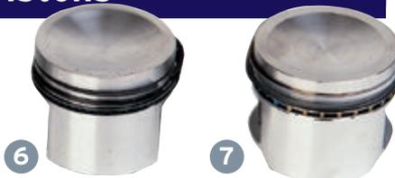
6. **The different CR's are achieved by different pin to crown heights, with 21.4cc cylinder head camber size.** The P21253 pistons are the best suited to high performance use, with a much smaller oil drain slot behind the oil control ring, thereby reducing the possibility of breakage.
