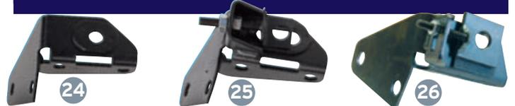
24. Pair of rear camber brackets to give extra 1/2° negative camber over the standard setting ..... **MS69**
