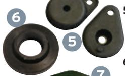
5. Front tear drop mounting on front subframe.
