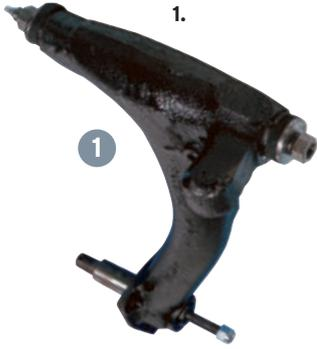
**1. Radius arm for vehicles with dampers** (known as dry suspension shock absorbers). Complete with pins and necessary parts ready to fit.
