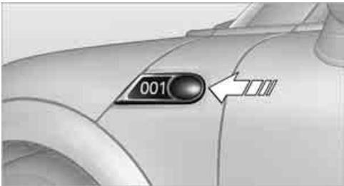
2. Screw out the bulb holder counterclockwise.
