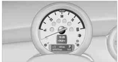
The display shows the percentage to which the high voltage battery is charged.
