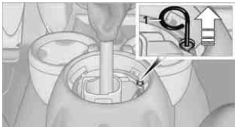
3. Take the hub cover remover 1 out of the glove compartment and insert it in the loop on the front passenger side.
