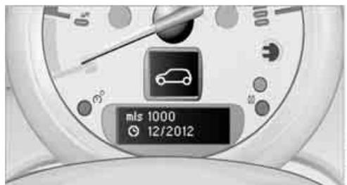
The remaining driving distance and the date of the next scheduled service are briefly displayed immediately after you switch on run position or the ignition.
