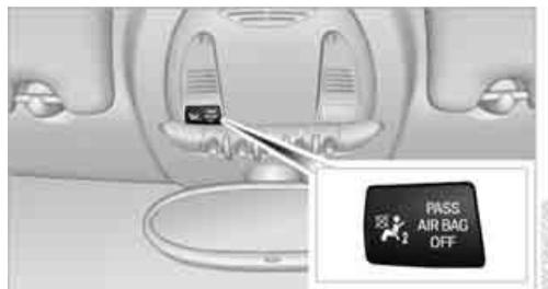
The indicator lamp for the front passenger airbags shows the functional status of the front passenger's front and side airbags in accordance
