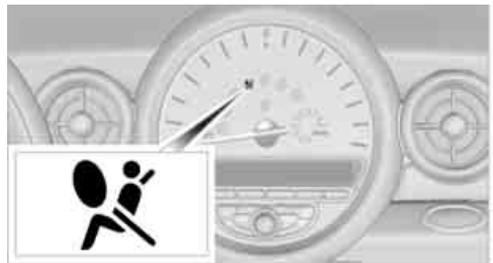
Beginning with the accessory position, page 32, the warning lamp comes on briefly to indicate that the entire airbag system and the belt tensioners are operational.
