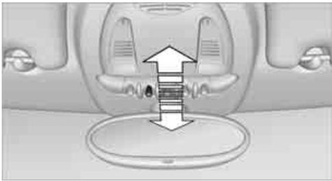
To switch the interior lamps on/off.
