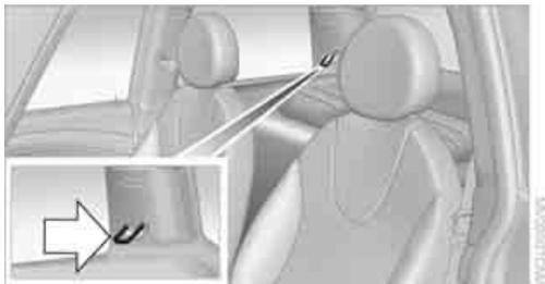
There is an additional anchor for child-restraint systems with a tether strap, arrow.
