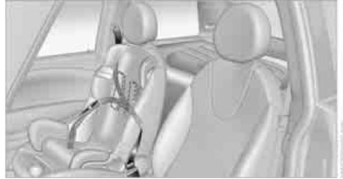
The safety belt for the front passenger can be locked to prevent it from being pulled out when it is used to secure child-restraint systems.
