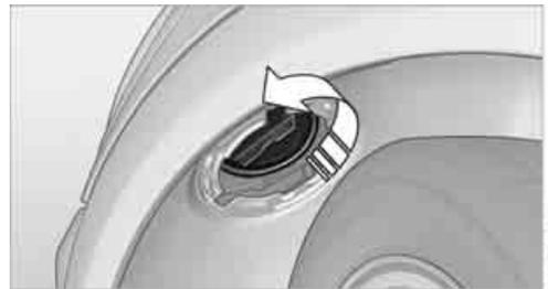
4. Screw out the bulb counterclockwise.
