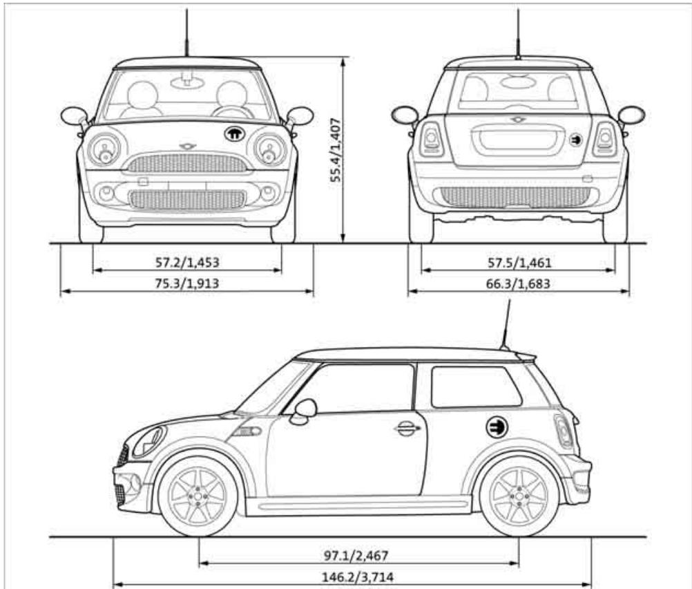
All measurements in inches/mm. Smallest turning circle Ø: 35 ft 10 in/10.7 m.
