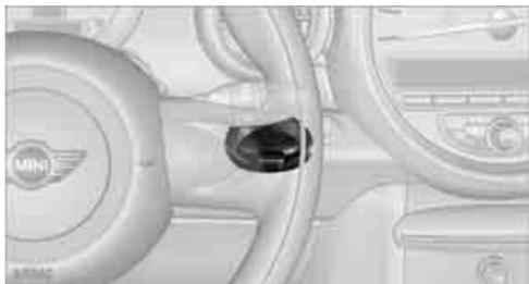
Insert the key all the way into the ignition lock: The accessory position is switched on and individual electrical consumers are ready for operation.
