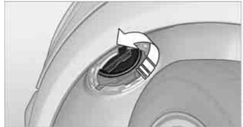
4. Screw out the bulb counterclockwise.
