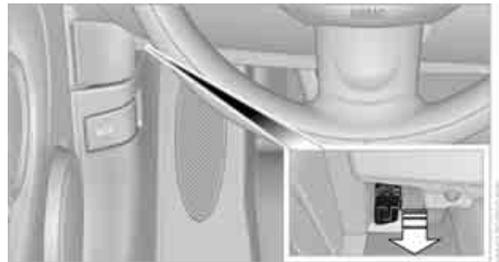
This socket is located to the left of the driver's side, on the bottom of the instrument panel.
