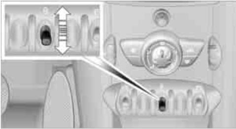
The switch locks or unlocks the doors and tailgate when the doors are closed, but the anti-theft system is not activated. The charge socket door remains unlocked\*.
