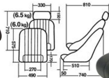
Fixed back traditional bucket seat. A low cost, entry level bucket seat, styled and constructed in a traditional manner. Deep sides and a low back ensure good comfort and support without the restrictions of a larger seat.
