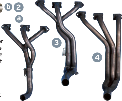
All Long Center Branch Manifolds have Y piece and gearbox clamps.
