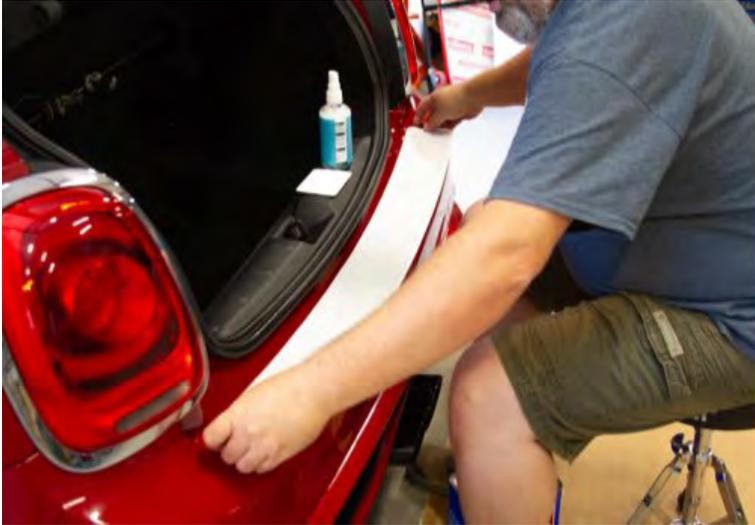
4. Once you're pleased with its positioning, start from the middle and gently squeegee the soap/water solution out from under the decal. Use paper towels to clean up any excess solution while you work the decal down.
