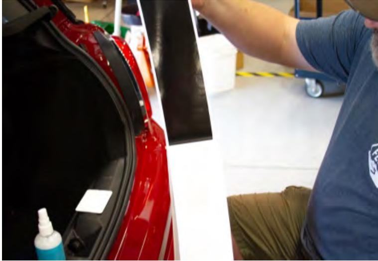
2. Take your utility bottle and spray an even coat of your soap/water solution to the adhesive side of the decal. It doesn't need to be completely soaked... it just needs enough for you to be able to readjust the decal if you don't set it down perfectly straight on the first try. Spray some of the soap/water solution onto the top surface of your MINIs bumper as well.
