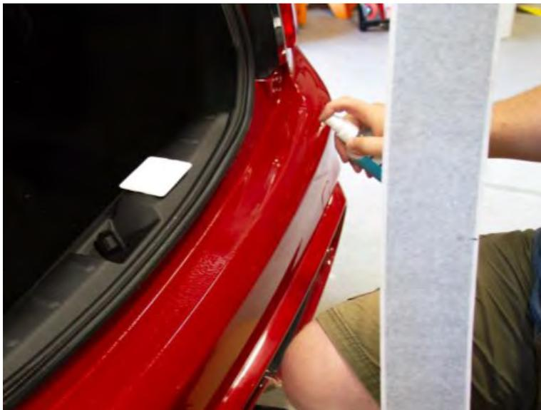
3. Hold the decal outstretched with your hands on either end and gently set the decal down onto the bumper surface, again lining up the center mark with the center of the bumper. The soap/water solution should give you the ability to either pull the decal up again or slide it around to line it up precisely.
