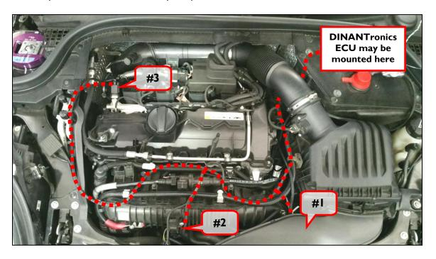
NOTE: There are two possible connector styles for Sensor #3. You may wish to glance at steps 11& 12, to confirm that the connector on the Dinan harness is correct for your vehicle, before continuing with this installation.
