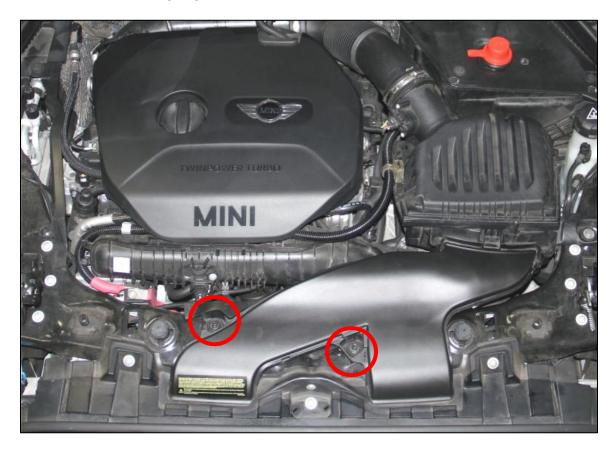
5. The charge air tube pressure sensor is shown below. It will have a connector that is identical to the ones on the DINANTronics harness.
