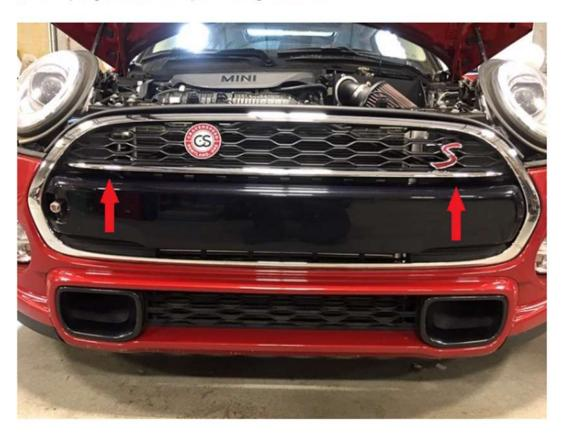
5. Grab a bracket in hand and enter behind the grill, placing the light mounting tab through the slot below the grill. The four-holed mounting portion of the bracket should lie flat against the v-brace core support bar.
