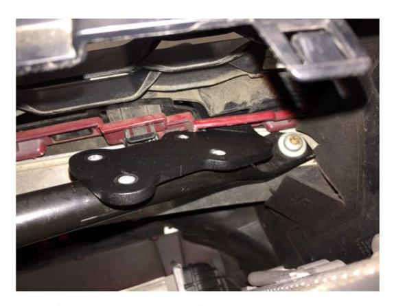
6. Insert the 1/4-20 x 1.25" stainless cap screws through the bar mounting portion of the light brackets with the cap heads facing up. Place the 'dog bone' shaped clamp on the backside and tighten the cap screws evenly with your 3/16" hex key wrench. Ensure that the light mounting tabs that come through the slots under the grill are level before performing a final tightening. Hand-tight is fine.. do not crush or deform the core support bars.
