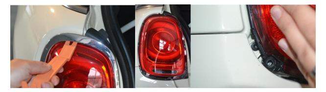
Remove the three T20 screws around the outer edge of each light. Pull off the trunk inside covers on each side. Unplug the tail light harness on each side and pull as far out as possible. To remove the tail lights pull gently, but firmly on the lower inside edge of the light housing. You can also reach in from behind the tail light and push on a clip near the lower inner side of the tail light.
