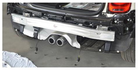
With the bumper removed, use a 18mm socket with extension to remove the 4 nuts that hold the aluminum support structure in place.
