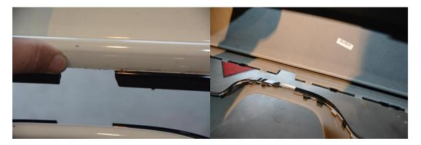
Reattach the mesh grill to the bumper, hang the bumper in place and test fit your drawbar to make sure it slides in and out freely. Trim any parts as necessary.
