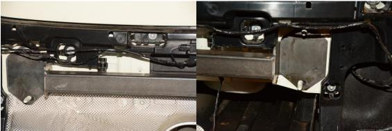
Reinstall the hitch on the studs and replace the aluminum bumper on top of the hitch. Tighten the four nuts to hold the bumper and hitch in place. Torque the 4 nuts to 17 ft/lbs.
