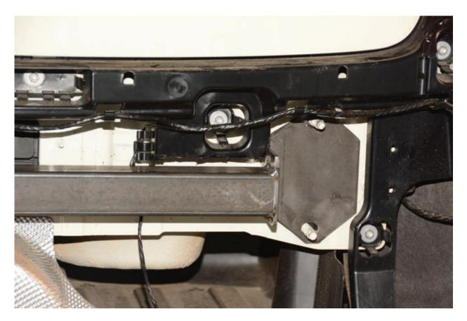
Inside the bumper are a series of tabs along the edge of the mesh grill where it connects to the bumper. Pry on these off one by one while pulling on the grill to separate it from the bumper.
