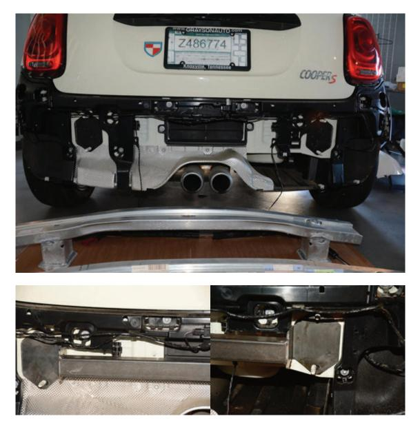
Reinstall the hitch on the studs and replace the aluminum bumper on top of the hitch. Tighten the four nuts to hold the bumper and hitch in place. Torque the 4 nuts to 17 ft/lbs.
