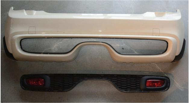
Once removed, mark a 1.25" section in the center of the grill. Cut the grill where marked and you'll end up with 3 pieces. The middle part (1.25 wide) will be discarded.
