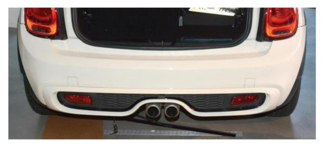
Trim (or bend out of the way) the soft metal heat shield with shears to allow access to the drawbar hitch pin from either side of the exhaust tips (behind the bumper) and roll the cut edge to keep it from causing injury.
