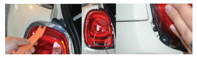
Remove the three T20 screws around the outer edge of each light. Pull off the trunk inside covers on each side. Unplug the tail light harness on each side and pull as far out as possible. To remove the tail lights pull gently, but firmly on the lower inside edge of the light housing. You can also reach in from behind the tail light and push on a clip near the lower inner side of the tail light.
