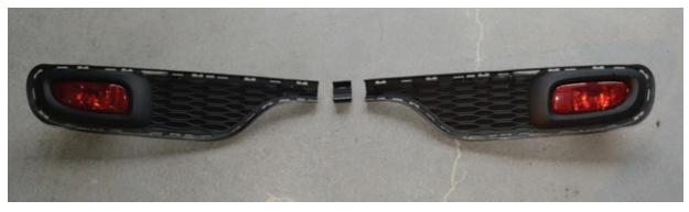
Next you will need to cut the glossy black trim that is attached to the bumper. It's best to use a a fine hacksaw or a dremel with cutoff wheel. Mark a 1-1/4" wide section on the top and lower trim and a small portion of the bumper as shown and carefully cut out as shown in the picture..
