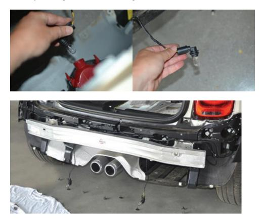
With the bumper removed, use a 18mm socket with extension to remove the 4 nuts that hold the aluminum support structure in place.
