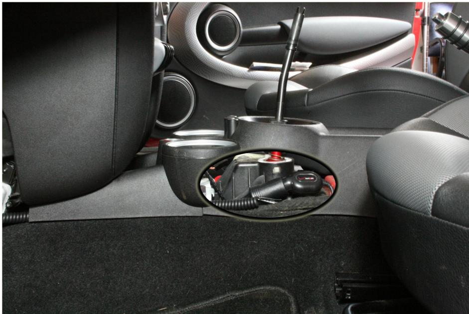
Reassemble the center console. Be sure to plug in your stock 12-Volt power socket! Next, replace the kick panel under the steering wheel. Finally, place your GPS or Smartphone into the clip and plug it in. Reconnect your car battery and turn the key on. The GPS or Smartphone should receive power normally.
