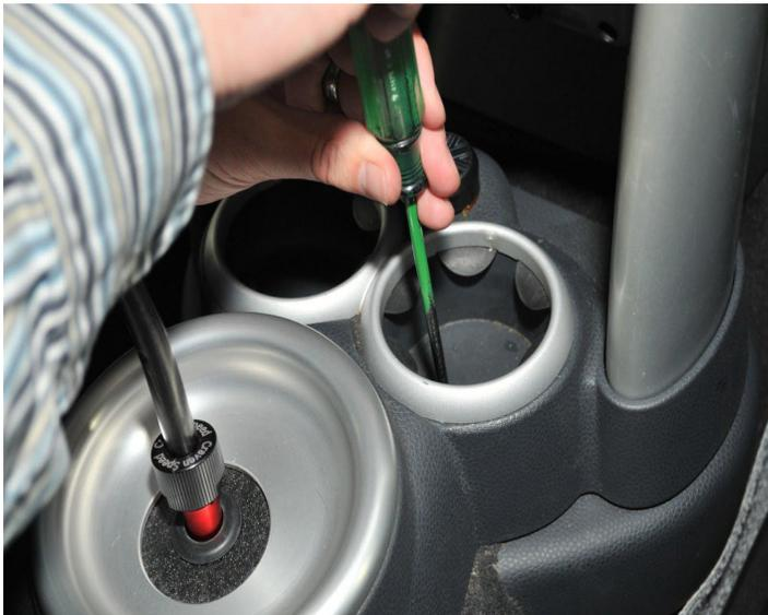
Carefully with a plastic tool or a screwdriver, pinch the middle of the sides of the emergency brake boot. Lift and maneuver the brake boot up, then the entire console can be lifted, but don't pull! The power wires to the 12-Volt socket are still in place.
