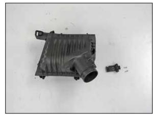
13. Remove the two bolts that secure the mass air sensor to the factory air filter housing and then remove the mass air sensor.
