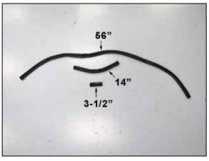
8. Cut the provided edge trim into three sections as shown. One section will be 56" long, one section will be 14" long, and one section will be 3-1/2" long.
