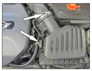
5. Loosen the hose clamp securing the intake tube to the air filter housing and unhook the ground cable from the air filter housing, then lift up the air filter housing and remove it from vehicle.
