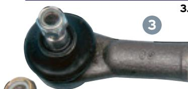
3. Longer track rod ends are for use on lowered cars or cars with negative camber where the original has insufficient thread for the standard rod end to screw safely onto steering rack. Also fits Midget and Sprite. Sold individually . . . . . **GSJ158**
